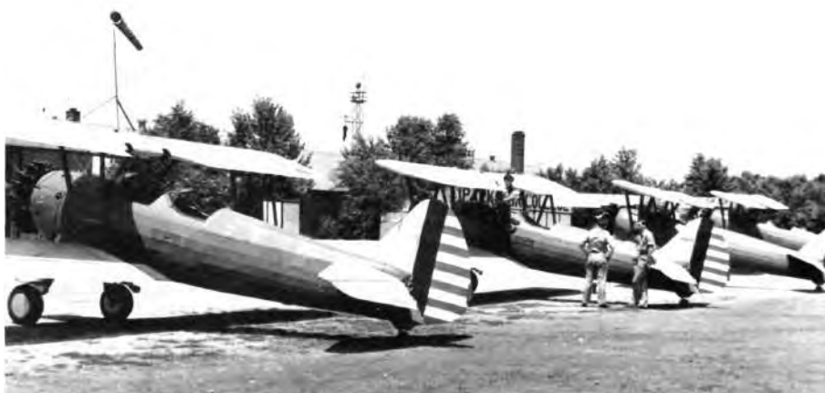
These 11 Stearman PT-13s are all prepared for flight at Parks Air College on May 28, 1940. The PT-13 was powered by a 215-hp Lycoming R-680-5 engine.
