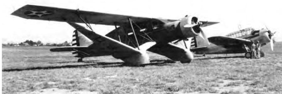
One of the more unusual visitors to Parks Air College was this Bellanca C-27A Airbus, one of 14 built for the Army Air Corps. It was powered by a 650-hp Pratt & Whitney R-1860 Hornet engine. In the background is a North American O-47 observation aircraft.
