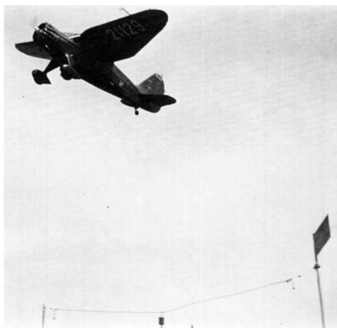
All American Aviation SR-10C using grapple system for pickup at Johnstown, PA, August 1940. (Earl F. Stahl)
