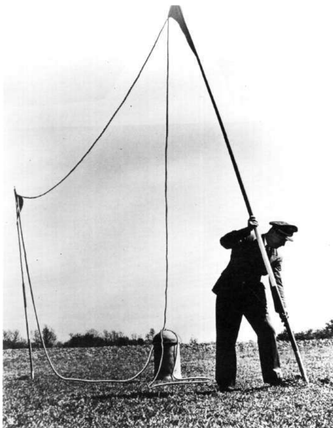
Aluminum tubing, bamboo-tipped pickup station poles were 12 feet tall (originally 20 feet). Wire clips on canvas flags held 3/8-inch nylon rope aloft. Protective container, 28.5 inches tall, rested on ground. (USAir)
