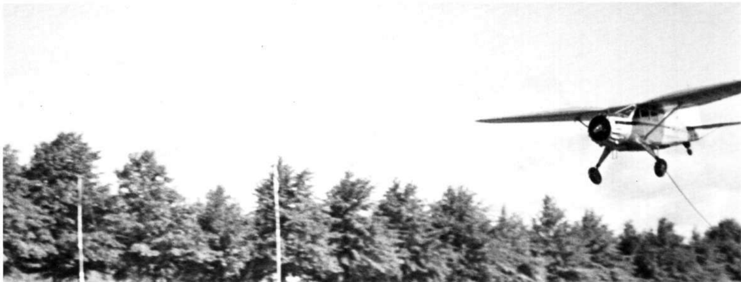
Stinson SR-10C's nimble control response enabled pilots to make pickups safely adjacent to trees, buildings and other obstructions in the frequently occurring low-level turbulence. (Earl F. Stahl)
