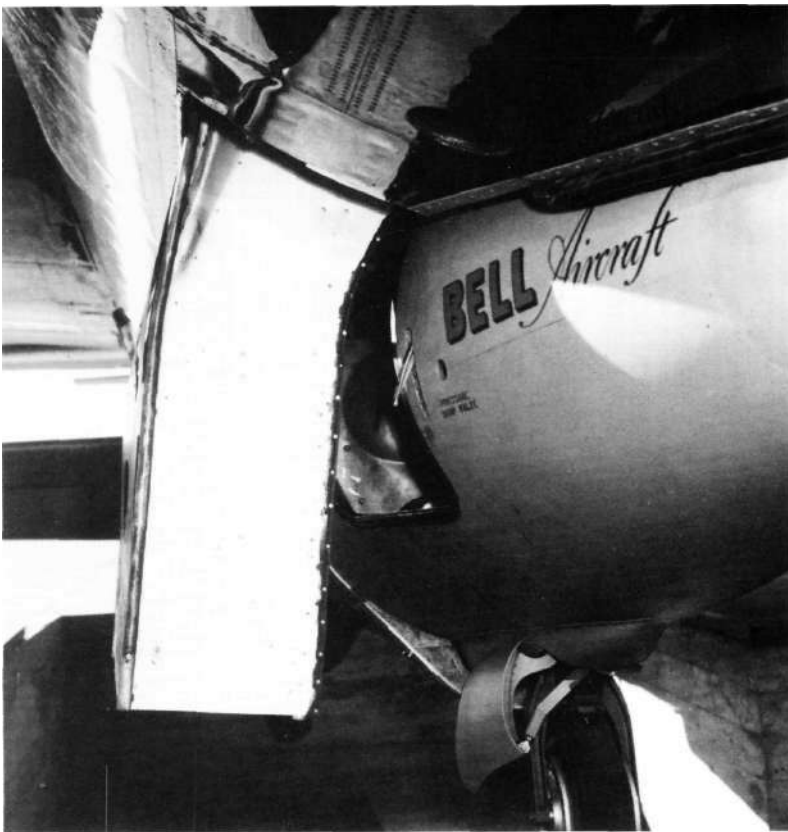
March 1947—During the climb to launch altitude, the XS-1 cabin pressure regulator malfunctioned causing the cabin pressure to exceed 1,000 feet below sea level. Consequently, it was necessary for pilot Chalmers Goodlin to jettison the entrance door which struck the access ladder with such force that it was bent outward making it inoperable and unsafe for Goodlin to attempt reentry into the B-29 mothership bomb bay. Therefore, Goodlin jettisoned all fuel and remained in the XS-1 during the landing at Edwards AFB.
