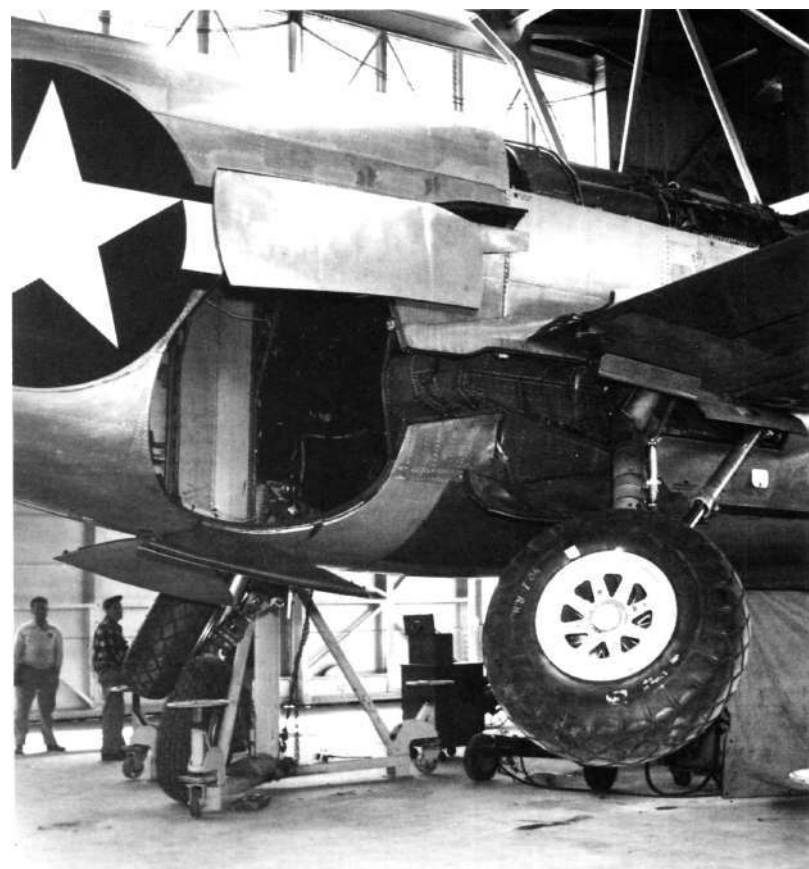
The long, complex main gear of the XB-43 folding aft into the sides of the short fuselage caused critical center-of-gravity problems.
