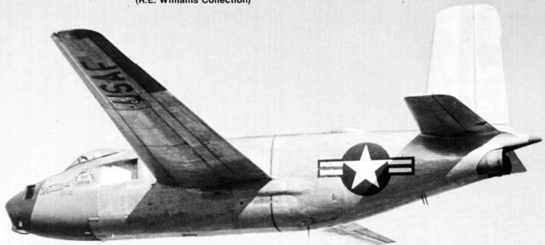
Ship No. 2 was modified for photo reconnaissance tests. Note camera ports in solid nose, and "Air Force Flight Test Center" logo. (R.E. Williams Collection)
