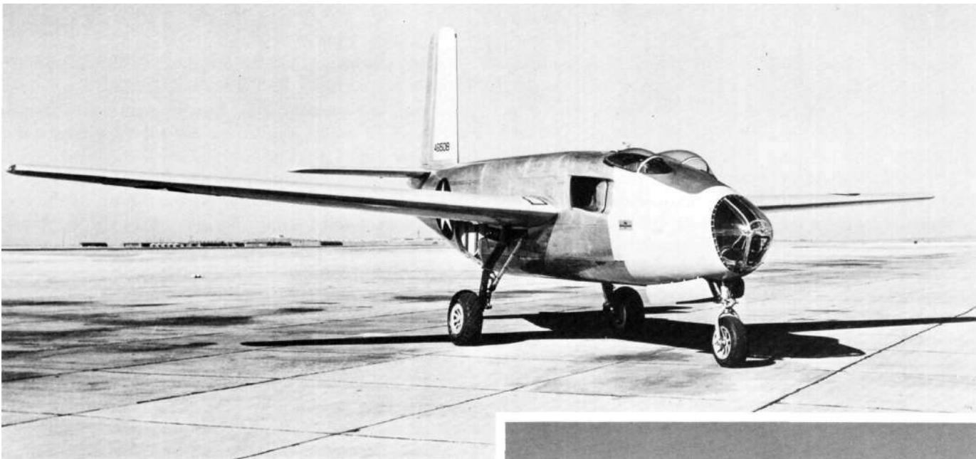
The clean lines of XB-43 No. 1 are evident in this front view at Muroc. The "bugeye" canopy was a flawed design giving both pilot and copilot a blind side and semi-isolation which inhibited communication.
