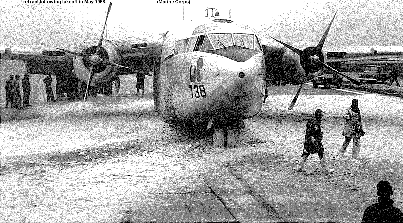
The crew of this VMR-253 R4Q-1, 128738, was forced to make a belly landing at MCAF Iwakuni, Japan, after the landing gear failed to fully retract following takeoff in May 1958. (Marine Corps)
