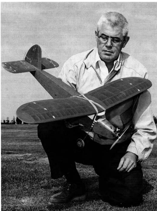
Winter with a Half-A powered radio control model being tested for a Scientific Co. kit in the early 1960s. It featured a single-channel radio with escapement to operate a rudder—the only control!
