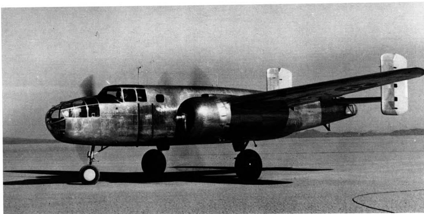
The first production B-25 (NA-62) with constant wing dihedral from root to tip and original fin and rudder shape. (North American Photo)
