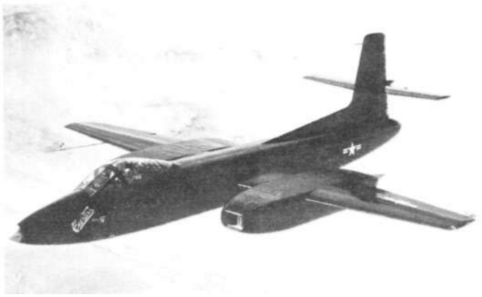
The Curtiss-Wright XF-15C-1 built in Buffalo and finished in Columbus. Shown here under jet power only with Lee Miller in the cockpit. September 3, 1946. Airplane flew at speeds up to 450 mph during tests of the T-tail. (C-W via Fred Steele)
