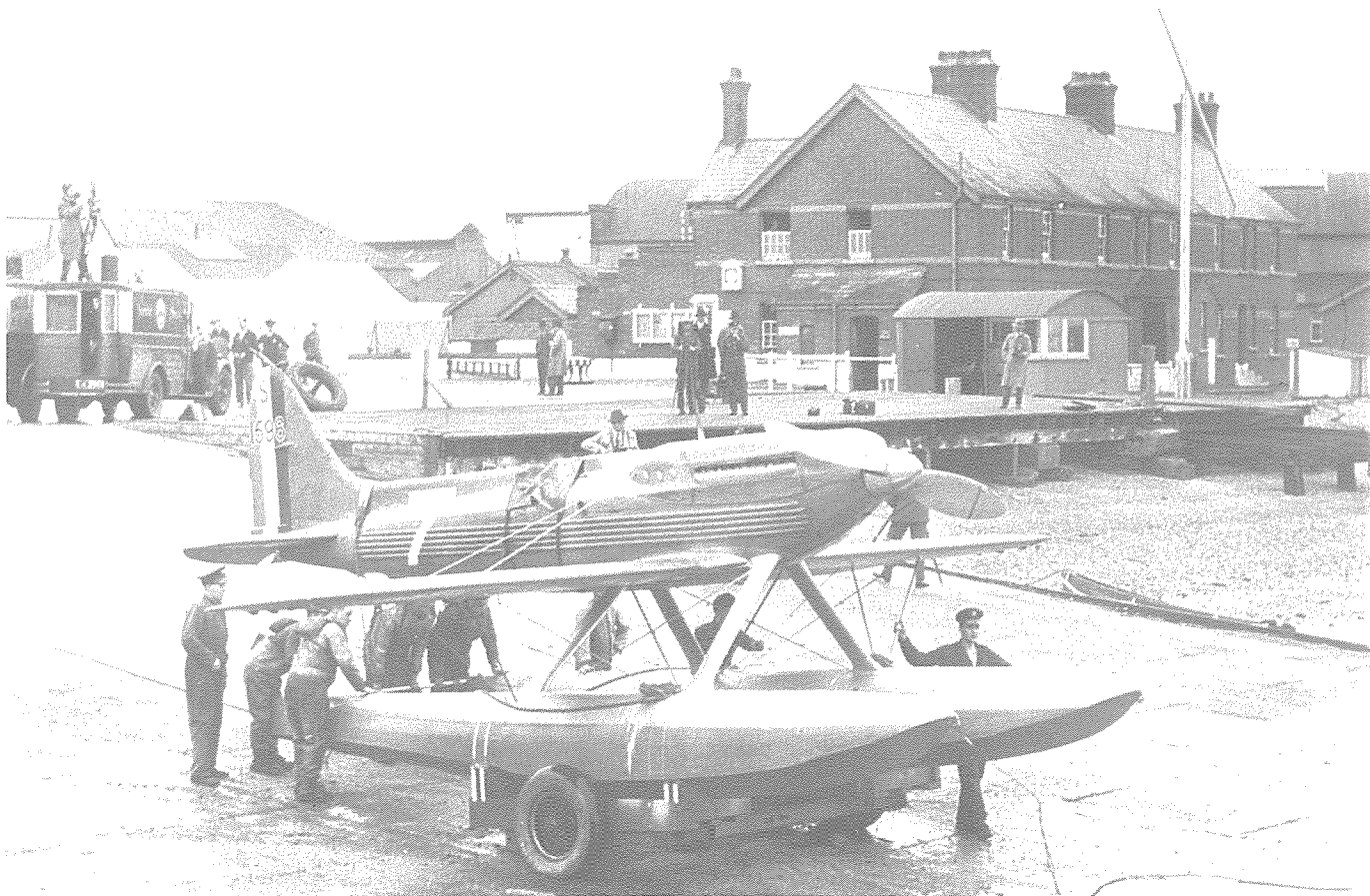
Supermarine S.6B S1596 of 1931 set the world's absolute speed record of 407 mph. To develop more power, fuel was changed to 30 percent benzol, 60 percent methanol and 10 percent acetone which allowed greater supercharging. (Unknown)
