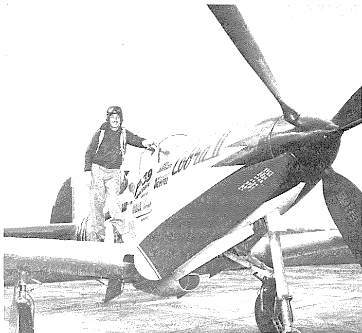
Bell P-39Q-10 Cobra II with pilot Tex Johnston onboard. Aircraft captured the 1946 Thompson Trophy Race. Photo shows the belly scoop oil cooler added to dissipate extra heat from race power operation.
