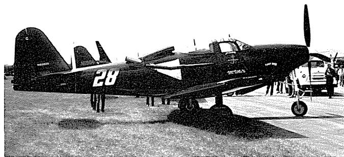
John Sandberg's beautiful red Bell P-63C-5 Kingcobra equipped with a dual Garrett turbocharger and setup to burn methanol fuel. Engine reliability problems plagued John and he reverted to aviation gasoline.
