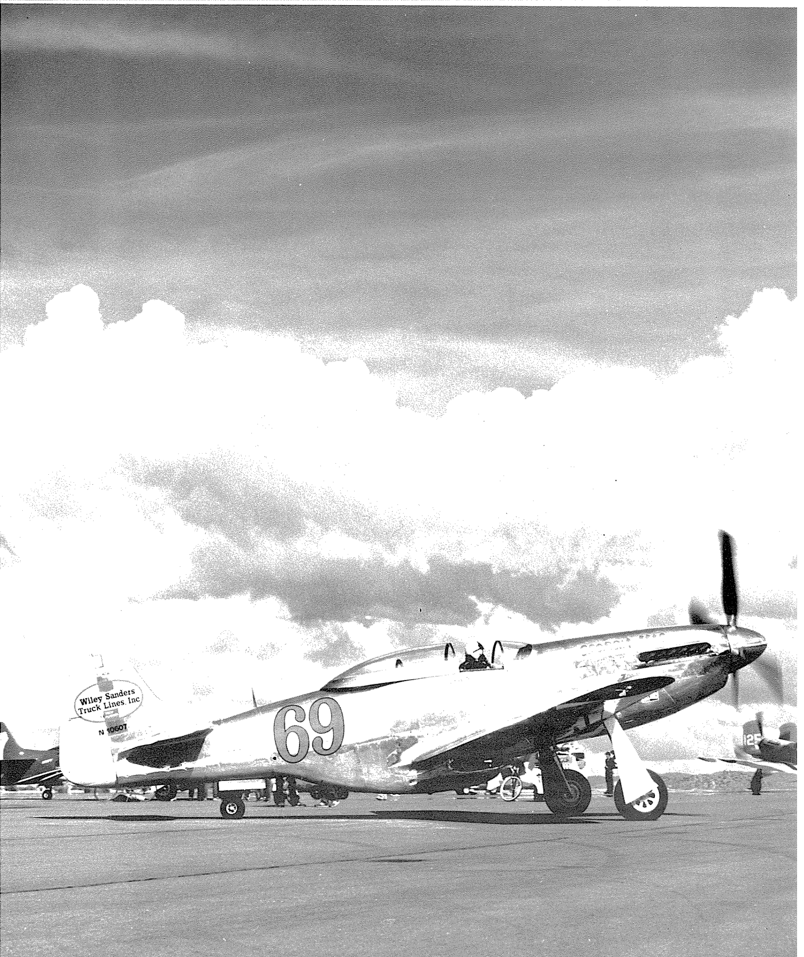
Although relatively stock in outward appearance, Wiley Sanders' Mustang has all of the current technology under the cowling including ADI and spray bars. The result is a serious Merlin -powered machine. (Birch Matthews)
