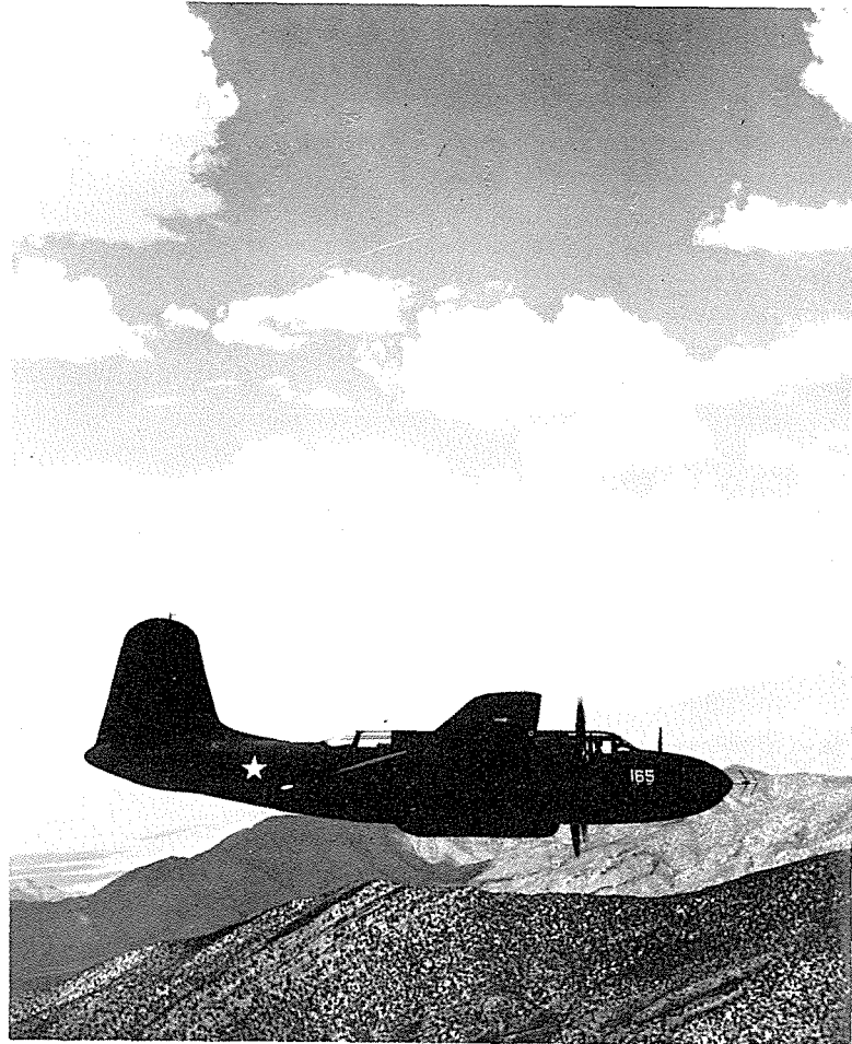
The 329 P-70s were night-fighter conversions of various A-20 models. Defensive armament was replaced by concentrated forward-firing guns and radar.
