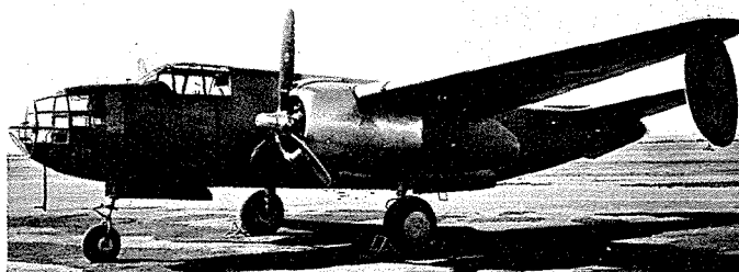
DB-7-131 was the only twin-tail version, produced at the request of the French to improve the field of fire. It was proven impractical by comparison tests with gun cameras, and was later changed back to a single-tail model.
