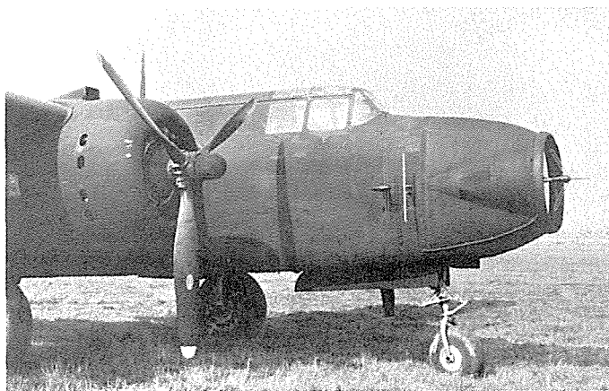
Closeup of a Havoc I Turbinlite nose modification. Twenty Havoc Is (converted French DB-7s) were supplemented by 39 Havoc II Turbinlite models converted from French DB-7As. (Author's Collection)
