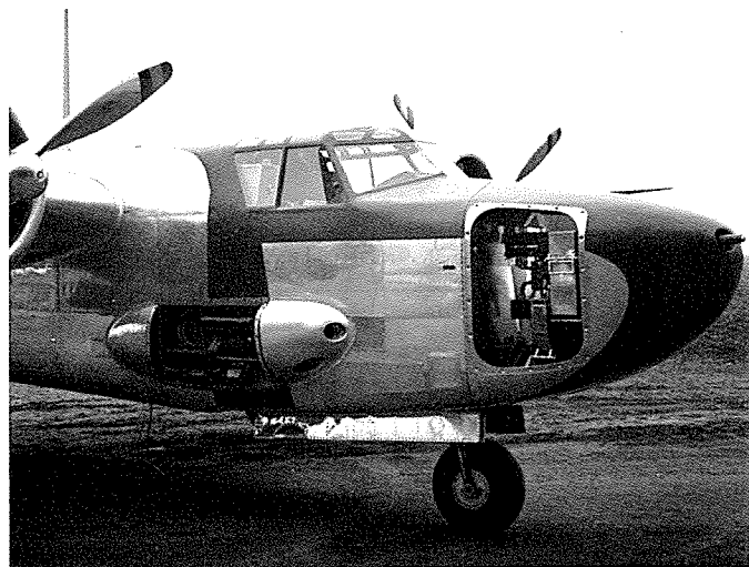
Closeup of the 7B with the attack gun nose installed and weapons service panels removed.
