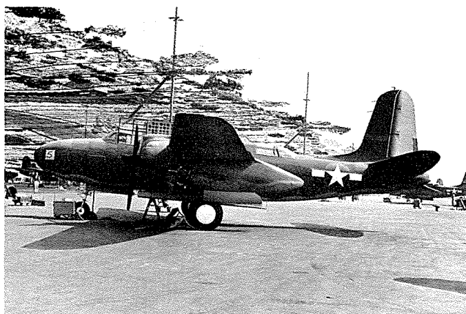
An A-20G-1 produced prior to rear turret installation effectivity. Note edge of camouflage netting which covered the wartime Santa Monica Douglas plant.
