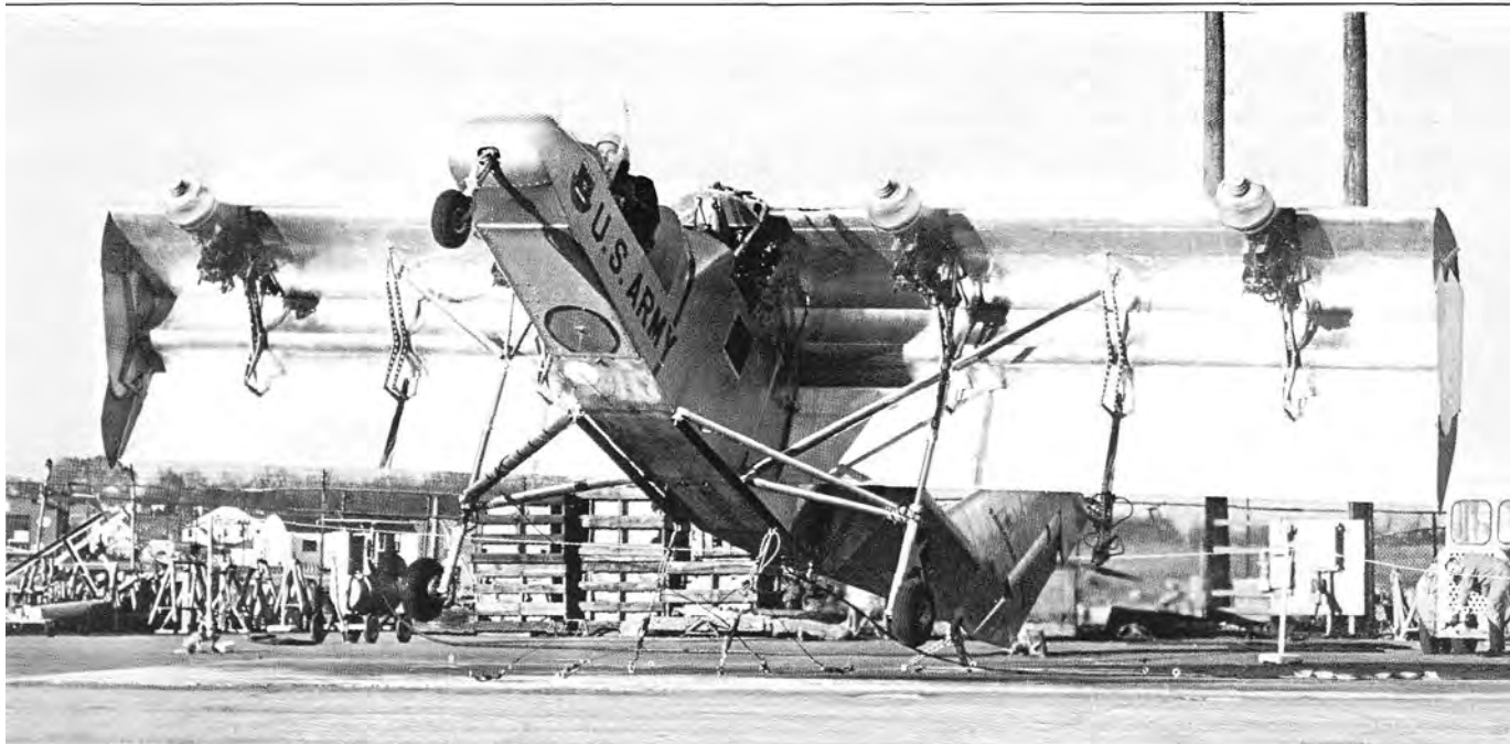
Altitude—18 inches! This is apparently the maximum height the VZ-5FA ever attained.
