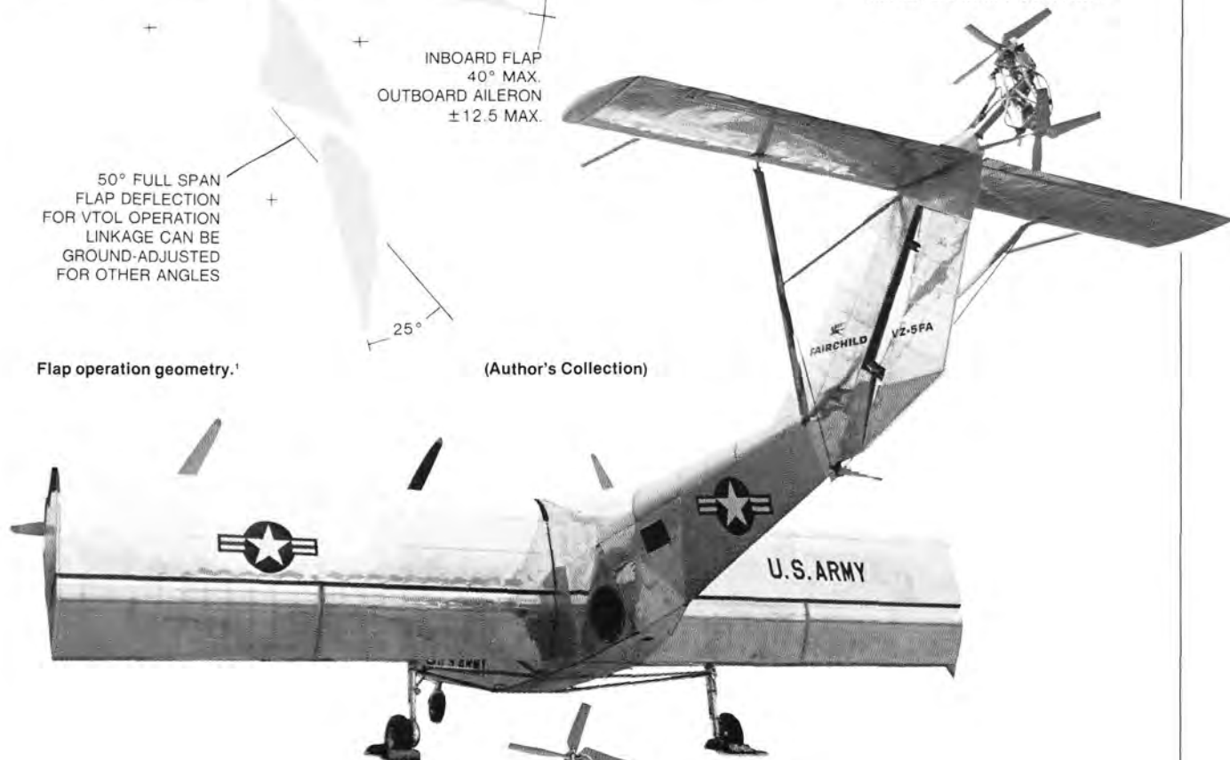
Three-quarter rear view, showing the T58 engine exhaust outlet and the hydraulic motor-driven, tail-mounted, pitch and yaw control fans. (Fairchild Aircraft Photo No. 35-88, Russell L. Howard Collection)
