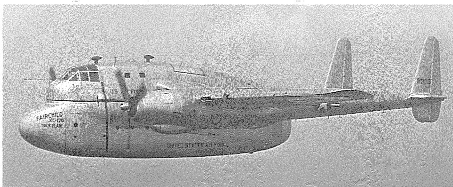
In-flight view of the XC-120. Note that the forward landing gear door needs some adjustment—it does not appear to be completely closed. (Fairchild Aircraft Photo No. 8-688)
