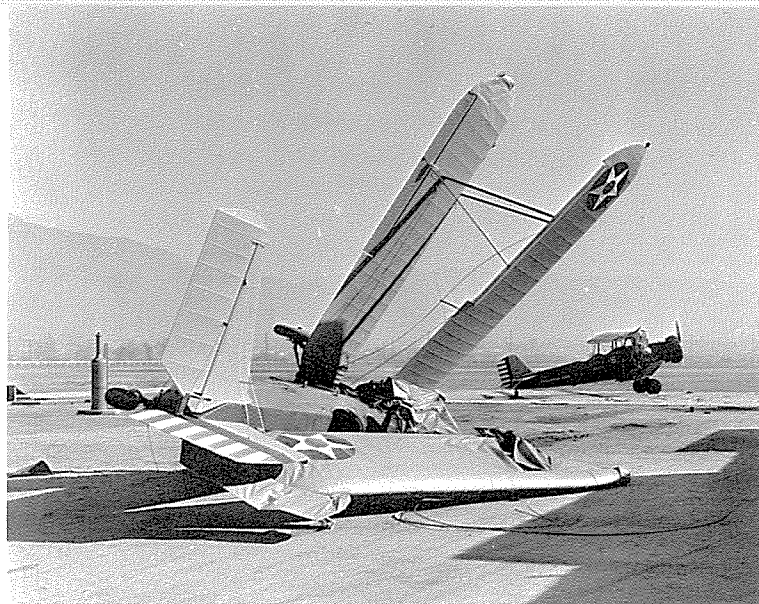
O-38B NG31-375 No. 7 in foreground with NG31-373 in background. Both show damage from the fog-shrouded collision earlier that day, 1 Feb. 1934.
