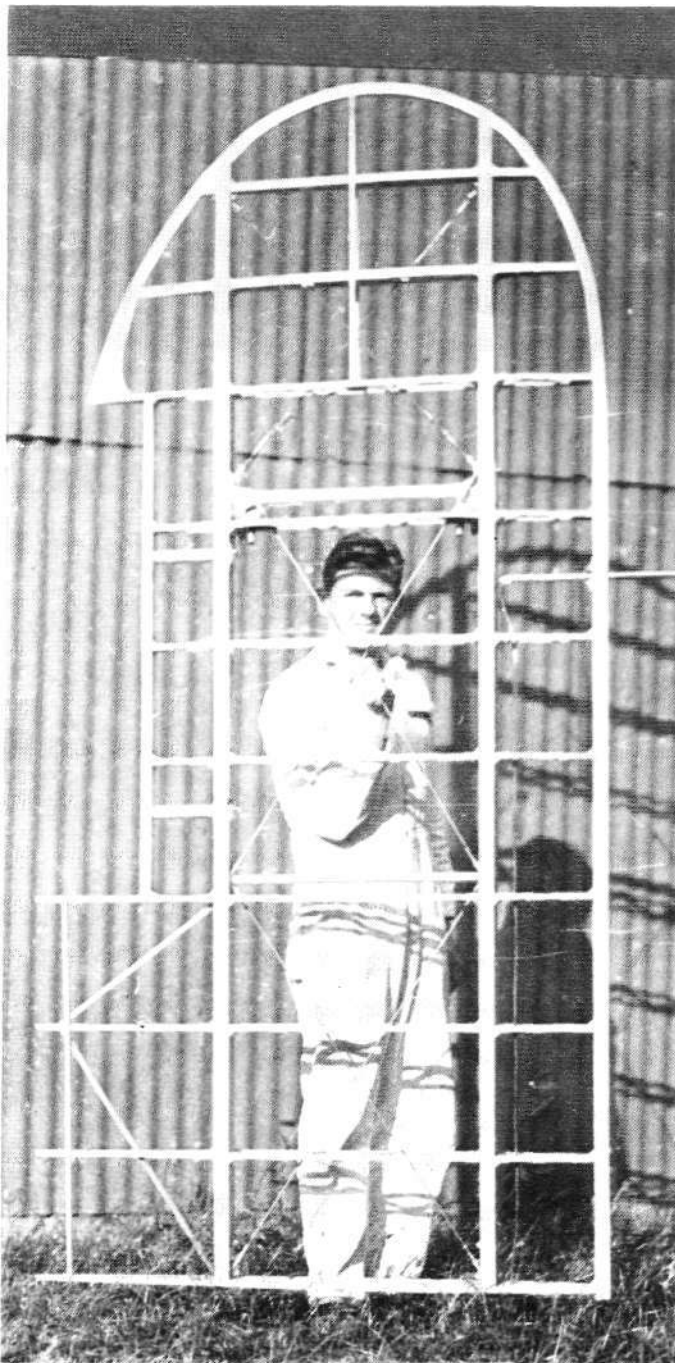
View of wing construction of the Model 22. This is a new wing and new airfoil, not just a clipped version of the We-Will Jr.
