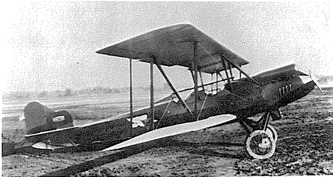
OX-5, 90-hp powered Lincoln-Page PT, NC-9415, which was a development of the LP-3 "Page Trainer." The Wedell-Williams Air Service owned three LP-3s, two purchased in 1928 and one in 1929 along with the PT. (Author's Collection)
