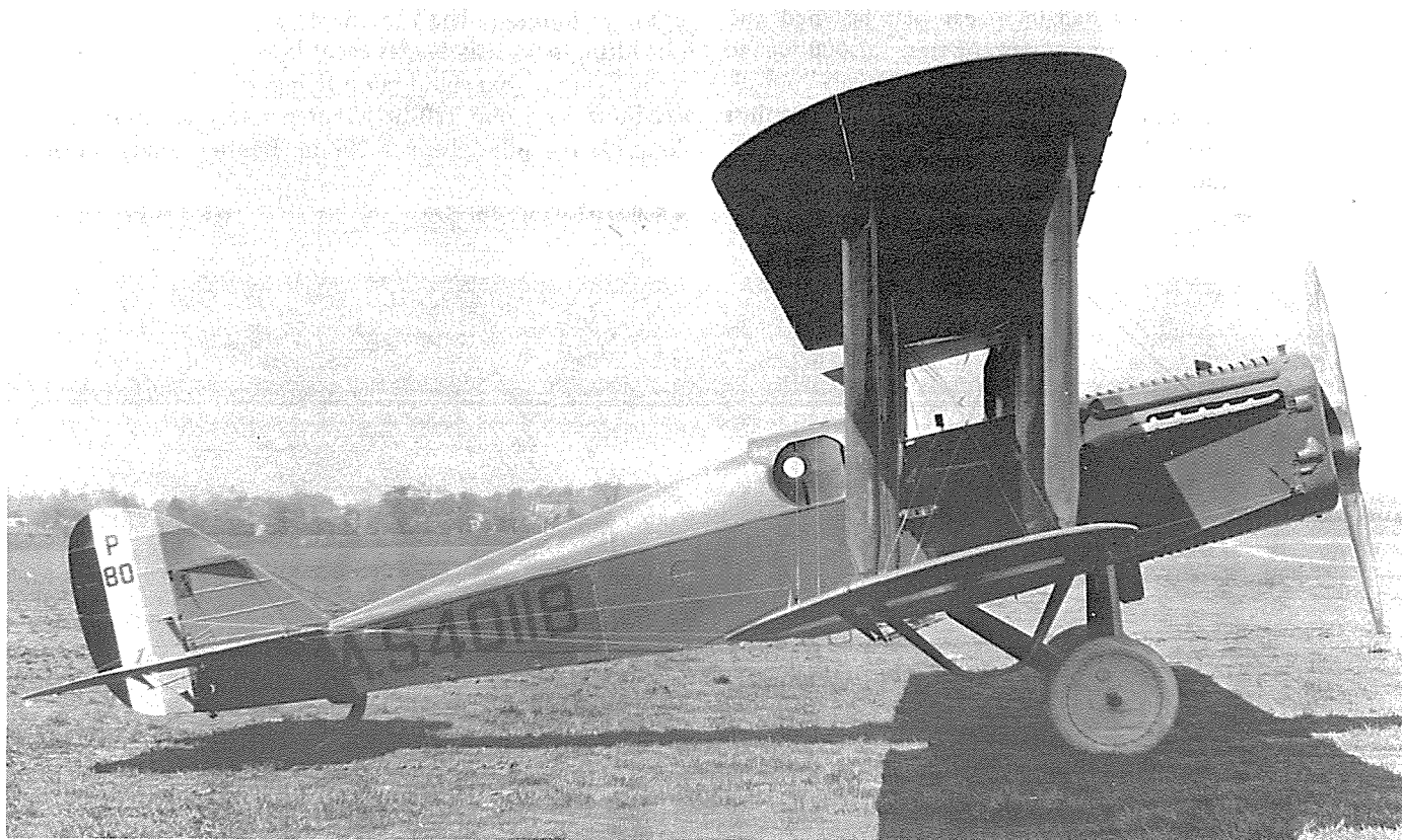
de Havilland D-9A, early experiment in pressurized cockpit, June 1921. (Peter M. Bowers Photo)
