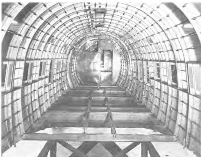
The secret of the DST/DC-3's durability lay in its basic construction of reinforced aluminum alloy ALC24ST. (Harry Gann DAC)
