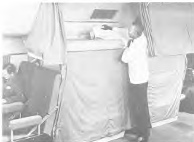
DST upper berth being made up. Note small, curtained slot window, characteristic of all DSTs. (Harry Gann DAC)
