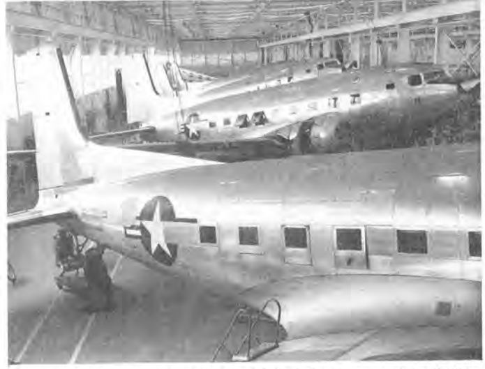
Douglas production line showing DC-3s being converted to R4D-8s, C-117Ds. (Harry Gann DAC)
