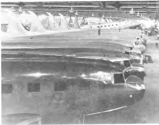
A DC-2/DC-3 production line. The DC-2s are in the foreground with square windshield. The DC-3s are in the background. (Harry Gann DAC)
