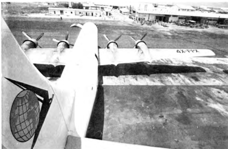
A wide-angle view of 4X-FPX showing the side loading door fitted to all the B-377s in IDFAF service, and enabling a close look at the squadron's insignia. (Author's Collection)
