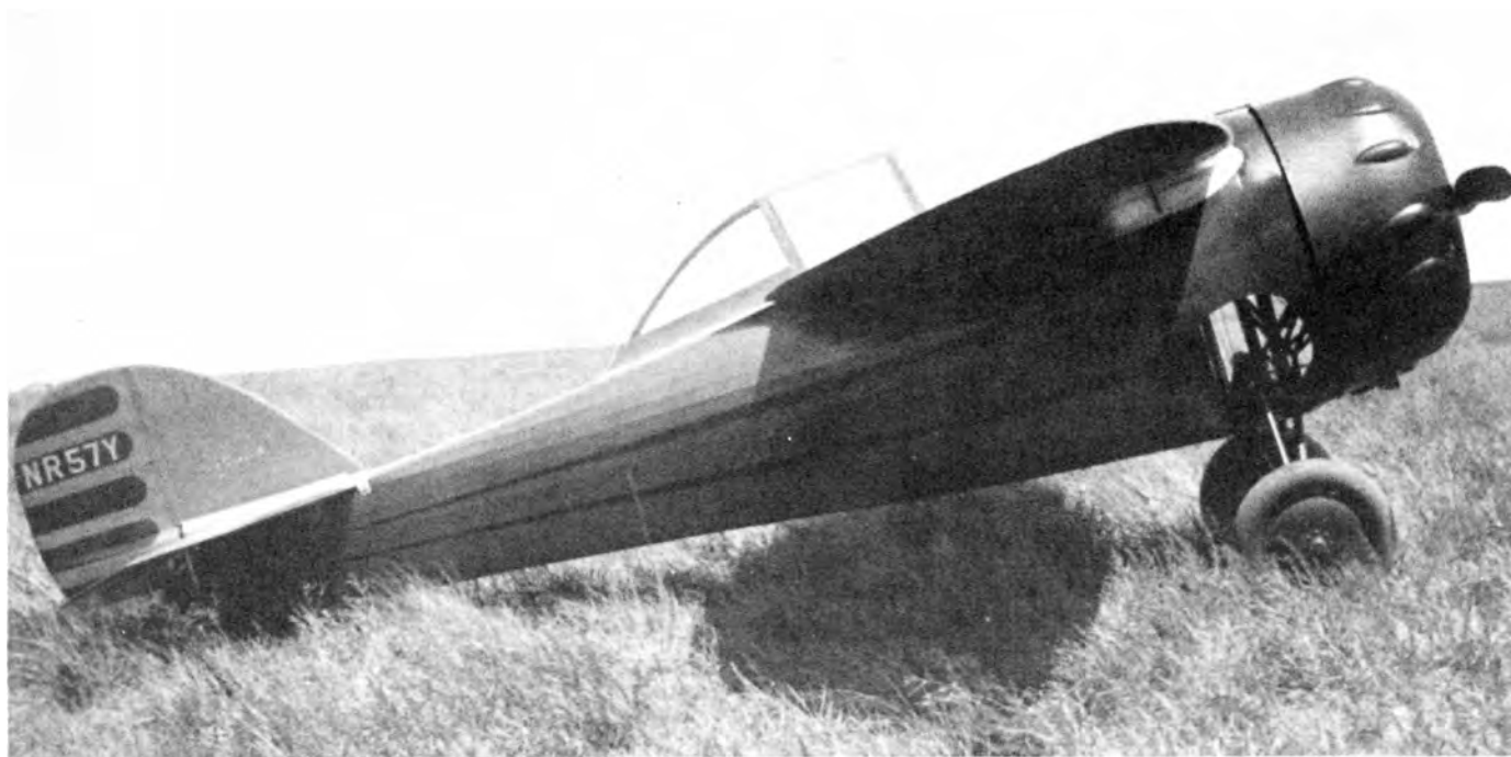
Side and front view of the Cessna CR-3 of John Livingston. This is original configuration with canopy. Note cylinders are baffled.
