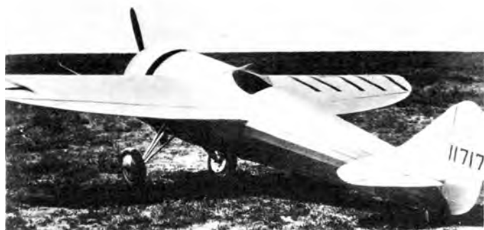
Cessna CR-2 as first flown by Eldon Cessna. This is a stretched version of the CR-1 which was about 2 feet, 8 inches shorter. It is not known if the CR-1 actually flew or was redesigned during construction. There are no public photos of it.
