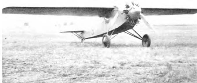
Cessna design No. 2 used for racing. Only one was built and was powered by early Wright engine.
