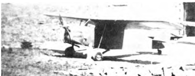
Cessna Cirrus-powered FC-1. This aircraft was owned and flown by Eldon Cessna. Only one was built but the wing, engine and empennage design was used on the GC-1 racer.
