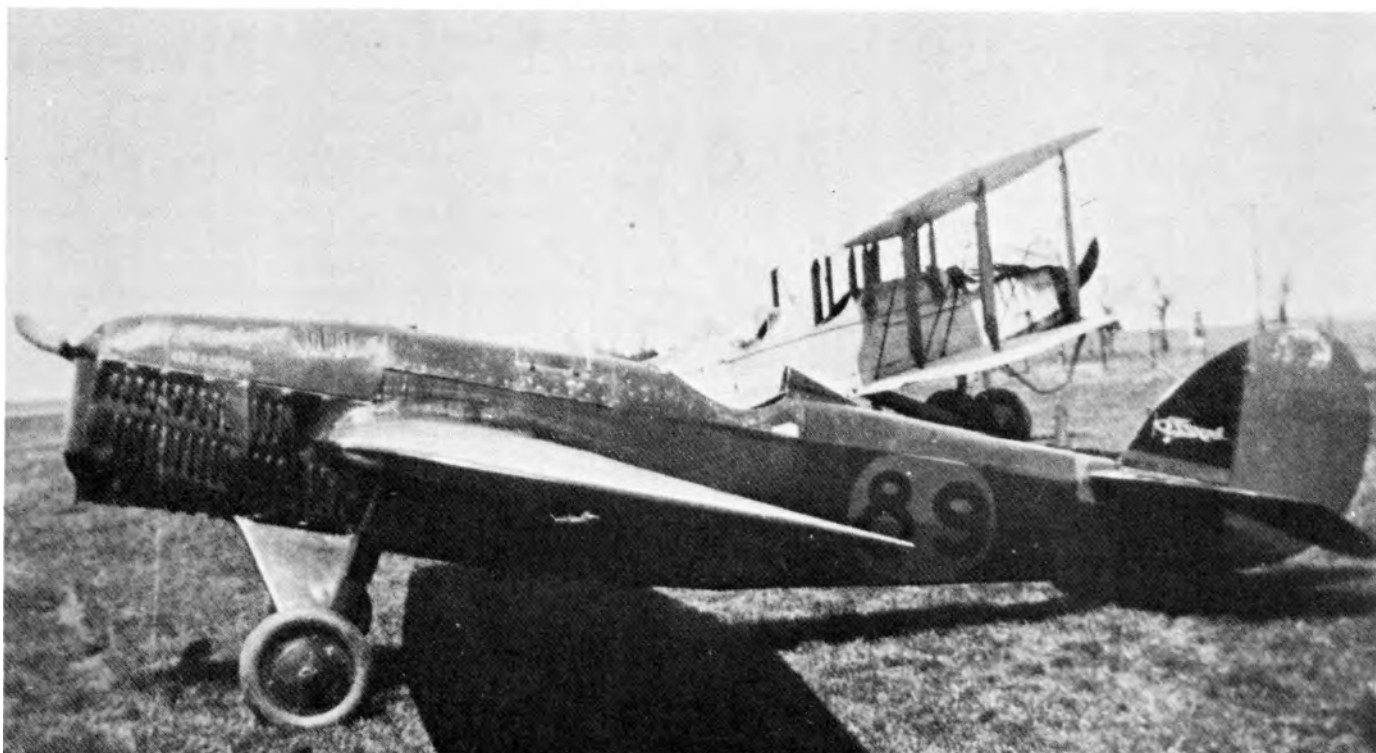
Cessna GC-1 after the 1930 National Air Races, with new race number and chin inlet to carburetor.
