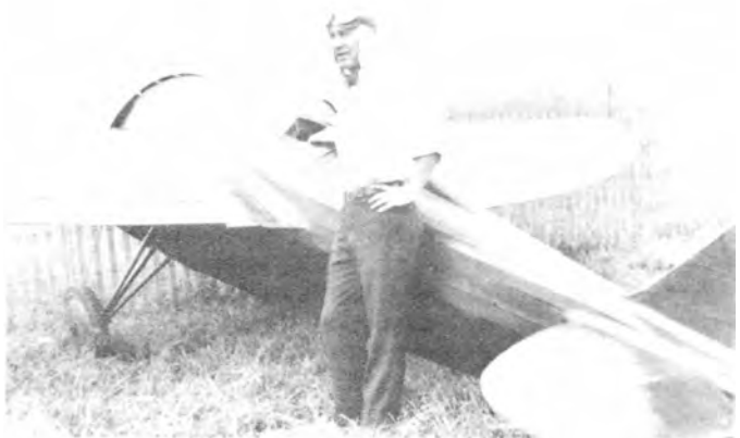
Roy Liggett standing beside his CR-2 shortly after taking delivery. Note the almost full-span ailerons. Roy was killed in this ship. He had installed a larger engine and improved the streamlining. It was bought and modified by R.O. Herman and called CR-2A.
