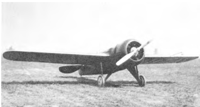
Cessna GC-1 after the 1930 National Air Races, with new race number and chin inlet to carburetor.
