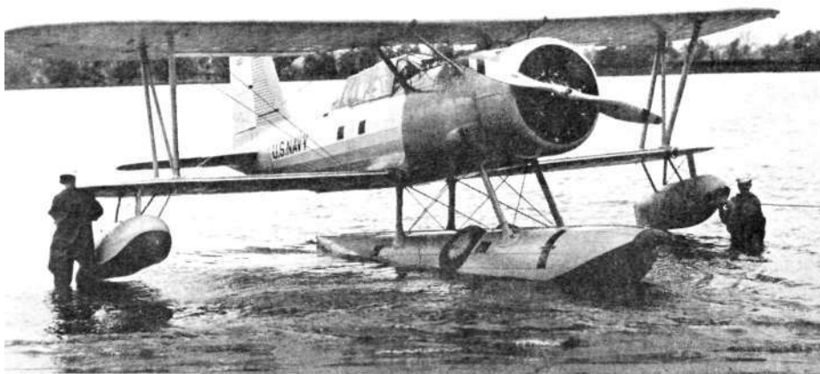
The XO2D-1 seen pulled up to the beach at Anacostia during amphibious trials. Mooring rings attached to the nose of each outrigger float facilitated handling. (MDC via Bob Williams)
