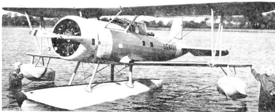
BuAer canceled the amphibious requirement during acceptance trials at Anacostia and tests were completed with plain floats. The XO2D-1 is seen on plain floats after repairs following the crash caused by a defective landing gear.
