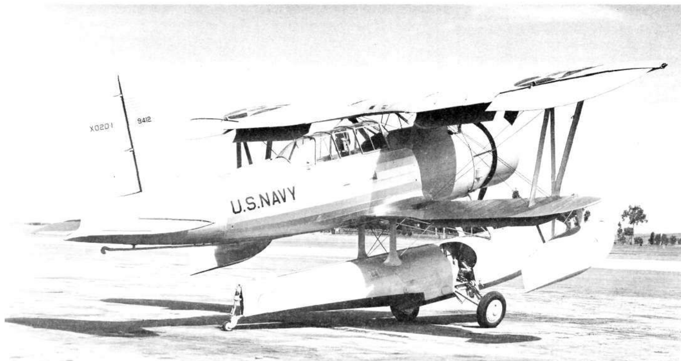
The XO2D-1, with lower surface flaps down and ailerons drooped 14 degrees, boasted full-span flaps. (MDC via Bob Williams)
