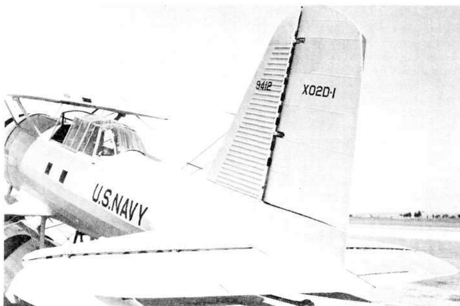
The elevators were reworked after the first flight to shorten the span of the trim tabs 40%. The two dark rectangles on each side of the fuselage by the cockpit are flush-covered recessed steps. The fuselage design looks very clean.
