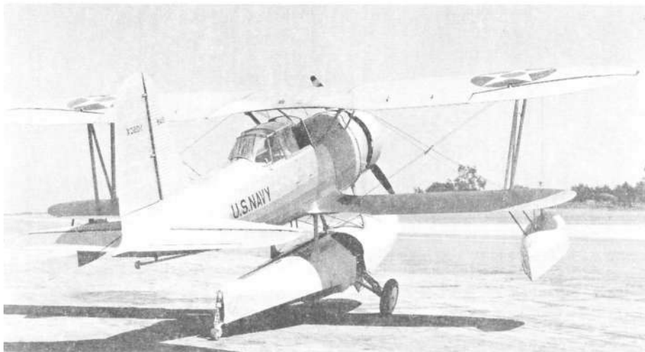
This view of the XO2D-1 shows some interesting design features. The lower wing chord was only about half that of the upper, and the aft fuselage was all metal. The center fuselage, like the wing, was fabric-covered metal frame construction. (MDC via Bob Williams)
