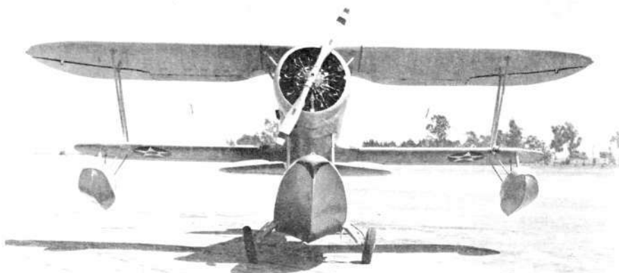
The XO2D-1 at Clover Field, Santa Monica, on the day of its first flight. Directional control while taxiing was difficult due to the narrow track of the main gear, a high center of gravity, and touchy brakes (later corrected). (MDC via Bob Williams)
