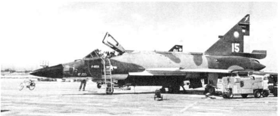
56-1163 being returned to flyable condition at Davis-Monthan AFB, June 1979. Note the new rudder. (Author's Collection via Ben Knowles)
