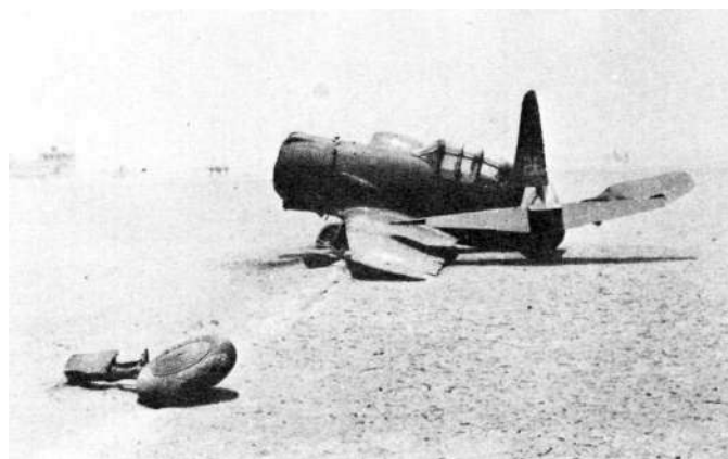
Fall 1942. Note Karachi Air Terminal in background. Taxiing B-17 and B-25 near terminal demonstrate that in the presence of a wreck, pilots simply landed around the accident. Timson comments that a lost landing gear leg often caused great destruction to airframe of crash-landed P-66s.
