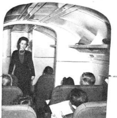
Interior view of the passenger cabin shows the clean lines and ample head room of the DC-5. The two main compartment partitions concealed the heavy structure supporting the wings in lieu of spars in the cabin area. (MDC)
