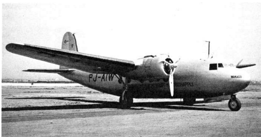
Wakago was shipped to Curacao, because of the war in Europe. Here it is shown ready for service. Note the addition of dorsal fillet and the new horizontal stabilizer configuration. (KLM)
