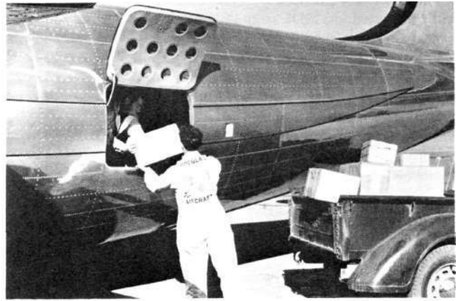
The low, level floor of the DC-5 made cargo loading fast and easy without the need for ground support equipment.
