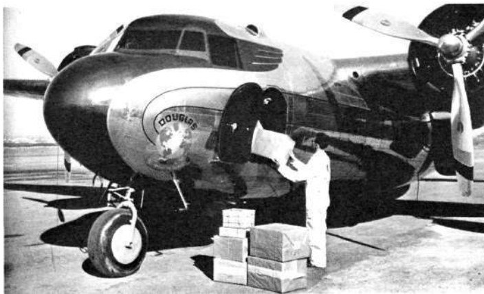
The low, level floor of the DC-5 made cargo loading fast and easy without the need for ground support equipment.
