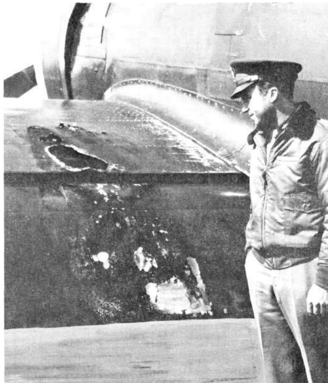
Damage to the Magic Carpet during her 42nd mission May 10, 1944. German 20mm anti-aircraft shell exploded in left wing knocking out wheels, flaps and left aileron and airspeed indicator. Hydraulic fluid caught fire and burned holes in wing. (Holt)
