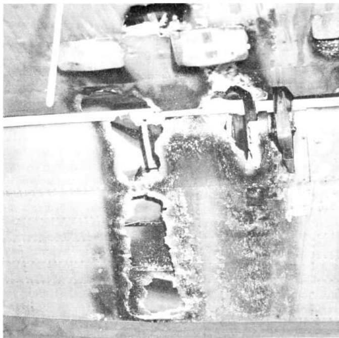
Damage to the Magic Carpet during her 42nd mission May 10, 1944. German 20mm anti-aircraft shell exploded in left wing knocking out wheels, flaps and left aileron and airspeed indicator. Hydraulic fluid caught fire and burned holes in wing. (Holt)
