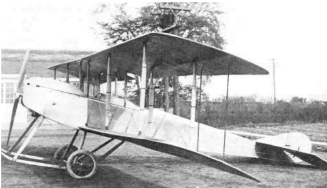
Mayo-Vought-Simplex biplane built for the British in WWI as a trainer. Mayo Radiator Works and Simplex Auto Company merged to go into aircraft production in war, with Vought briefly as chief engineer. This plane was rated excellent in flying qualities. Vought designed the plane in 1914 before the war had started. It was built in 1914. (Photo from Vought Albums)
