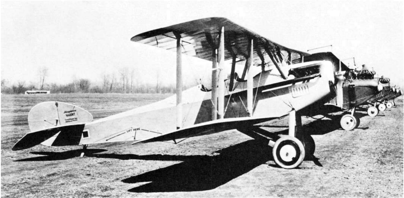
First plane, a VE-7, built by Lewis & Vought Corp., for the U.S. Army Signal Corps Air Service. Delivered to Hazelhurst Field, Long Island, Feb. 11, 1918, for entry in advanced trainer competition. Plane went to McCook Field, Dayton, Ohio, in March that year for flyoffs and won. Plane was built in 91 days, from contract award to completion. Note "Aeroplanes Vought" sign on vertical fin and small ventilation slits on side of nose. 150-hp Hispano-Suiza engine. JN-4s in rear. Hall-Scott engines' extended stacks.
