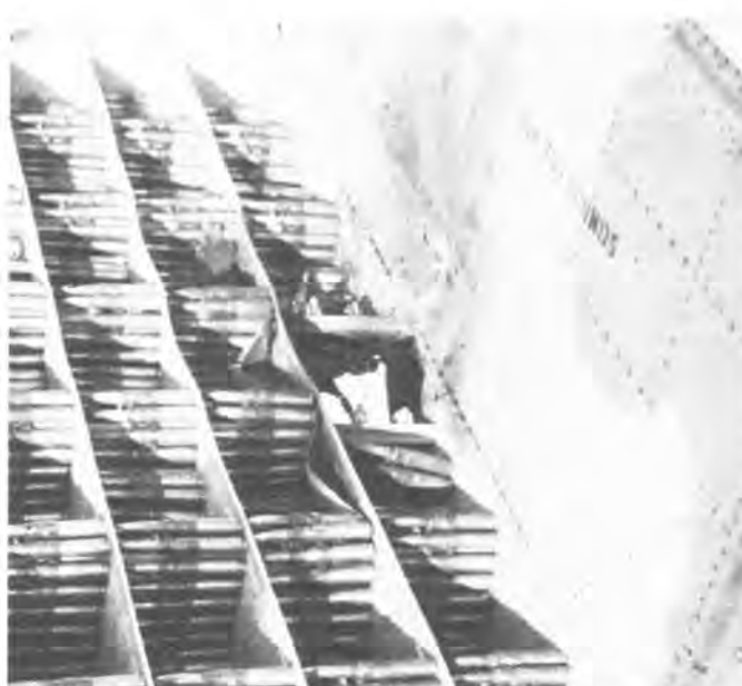
20mm shell hole in a .50-cal. ammo tray of a P-47, Mourmelon Le Grand, France. (Jack Robinson)
