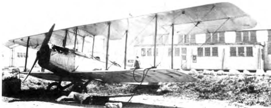
Hisso Standard J-1 with center section gas tank. Control and bracing cables show clearly. There were many varieties of J-1s due to so many types of equipment and accessories available for them, not to mention each individual modifying his/her ship to their preferences or available funds. 101-H was at Roosevelt Field No. 2 (west side), Mineola, on June 25, 1930. (Photo by DM. Ives)
