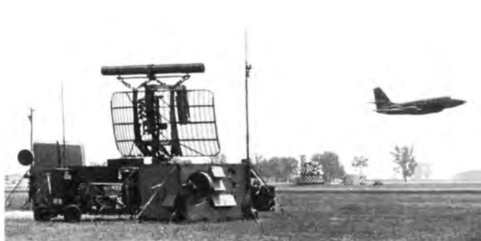
An 1866th Facility Checking Squadron C-140A makes a low pass over the Scott AFB, Ill., runway to check the TPN-19 landing control central. 1979. (Official U.S. Air Force Photo)
