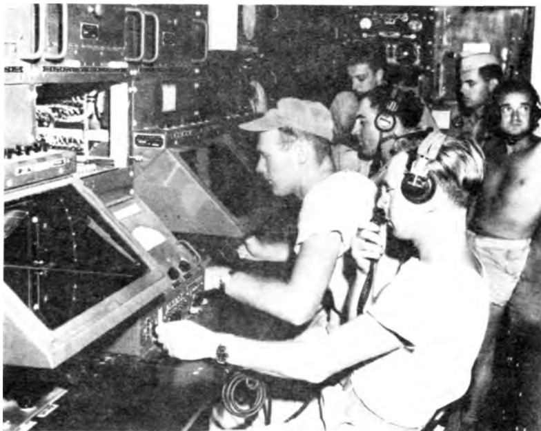
When bad weather cut visibility to a minimum, "Zippo," a precision radar, ensured a safe landing for aircraft arriving at Harmon Field, Guam, Marianas Islands. Operators are AACS men attached to the 20th Air Force.
