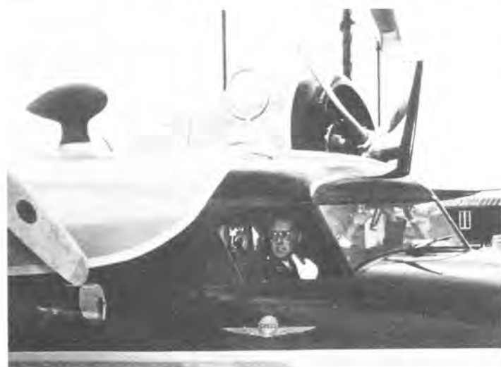
Prince Bernhard awaits start of PK-AKD's starboard engine as Shell pilot works throttles and starter. Overhead throttles and engine controls were standard on all amphibians to simplify control linkages. (Kavelaars Collection)
