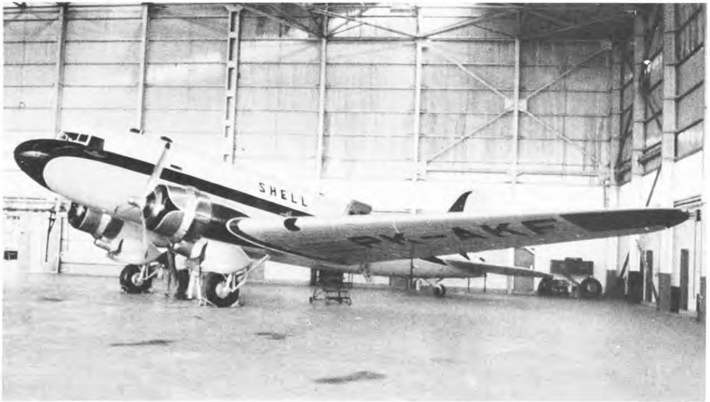
Shell's C-47A PK-AKF displays neat paint scheme as well as "Maximizer" kit installation (gear doors, tight cowlings). The first of four C-47s operated by Shell, AKF served from 1951 until about 1960. It was damaged in an air raid at Balikpapan on April 17, 1958, but rebuilt at Hong Kong. (Kavelaars Collection)
