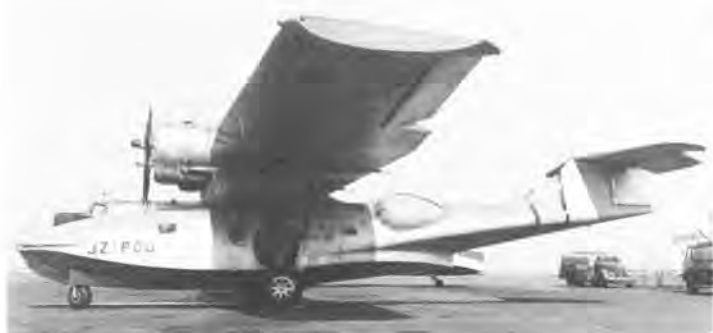
This 1958 photo at Oakland by Bill Larkins shows the last PBY, JZ-POD, en route to New Guinea. Standard nose, painted blister, "Rescue" stripe, and "PB-5AG" designation on fin betray its U.S. Coast Guard origins. Compare this with later photo of POD with JZ-POA. After arrival in New Guinea, "Clipper" bow was apparently fitted and blisters replaced with flush cargo doors. (William T. Larkins Photo/Kavelaars Collection)
