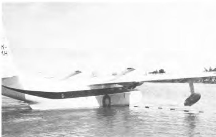
PK-AKH at Sanga-Sanga was operated by BPM at Balikpapan and carries a slightly revised paint scheme (note "Shell" on vertical fin). Torque from engines causes most still water taxiing to be done with the right float out of the water. (H.C. Kavelaars)
