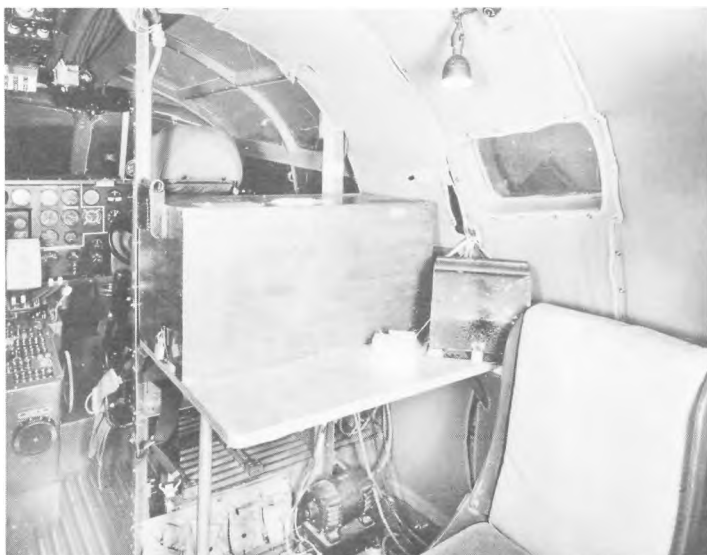
Part of the radio operator's station behind the copilot's seat on the flight deck. The table shown was to have carried the plane's radar controls and display when the ASG air-to-surface search radar was installed. Here it carries (locked) flight test recording instruments from the National Advisory Committee for Aeronautics (NACA). (National Archives 72-AC-66B-47/Consolidated 031-316)
