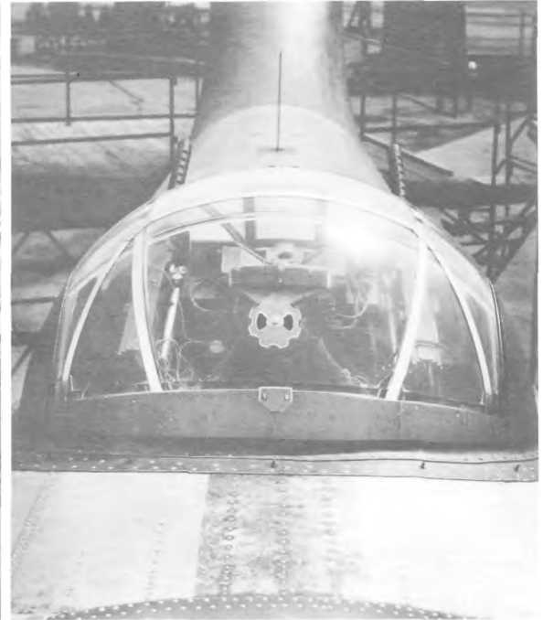
Exterior view of the ERCO 250SH mid-upper turret, looking aft from the escape hatch. The entire plexiglass top of the turret could be removed to provide an emergency escape route for the gunner.
