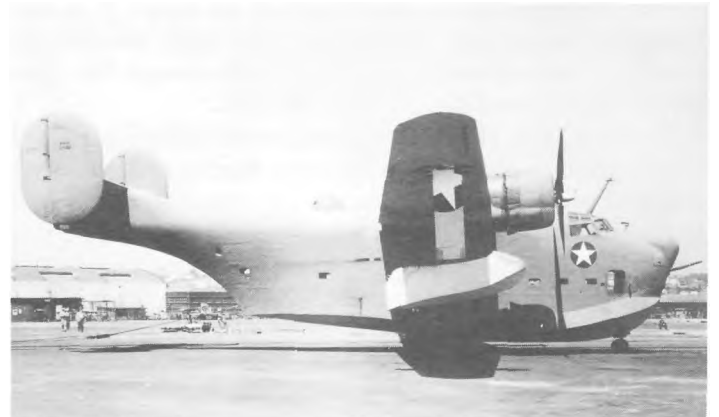
The XP4Y-1 in August 1943. Both forward mooring hatches are open, and the wing float shown bears a white coloring, as opposed to the sea blue on the rest of the upper and side surfaces of the aircraft. (National Archives 72-AC-66B-1)
