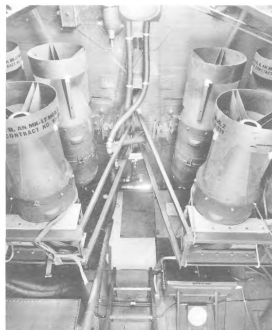
Bomb compartment on XP4Y-1, aft of the flight deck (note ladder and door to cockpit). Eight (unarmed) AN Mk. 17 Mod 2 325 lb. depth bombs can be seen; four are on the bomb carts, and four others are in racks below the wing center section. An alternate load was four 650-lb. Mk. 29 depth bombs. Additional bombs had to be hand-fitted to the bomb carts after the first were dropped. (National Archives 72-AC-66B-62)
