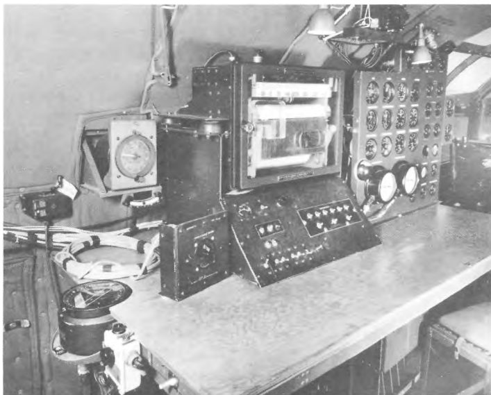
The navigator's table on the port side of the flight deck aft of the pilot's station; most of the equipment shown in this view is display and recording apparatuses for flight testing. An emergency escape hatch was located on this side of the flight deck, between the navigator's table and the rear bulkhead. (National Archives 72-AC-66B-44/Consolidated C31-319)
