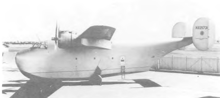
The Model 31 in its original configuration at the Consolidated factory in San Diego shortly after rollout in May 1939. Note the streamlined engine cowlings, straight fuselage spine.
