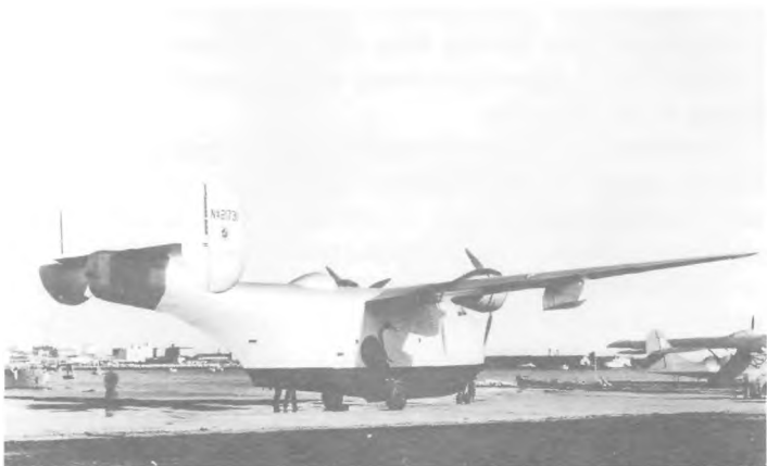
Another view in early April 1941, showing the outline of the proposed Consolidated tail turret, and the upper cupola blister turret.
