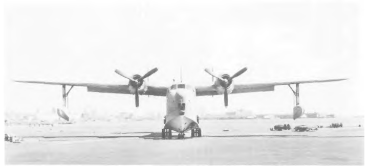
Head-on view taken August 18, 1943, at San Diego, showing extended wing floats, flaps, new Curtiss 16-inch diameter props, and conventional beaching gear. Although it weighed only two-thirds as much as the PB2Y, the P4Y was almost as big in its exterior dimensions.
