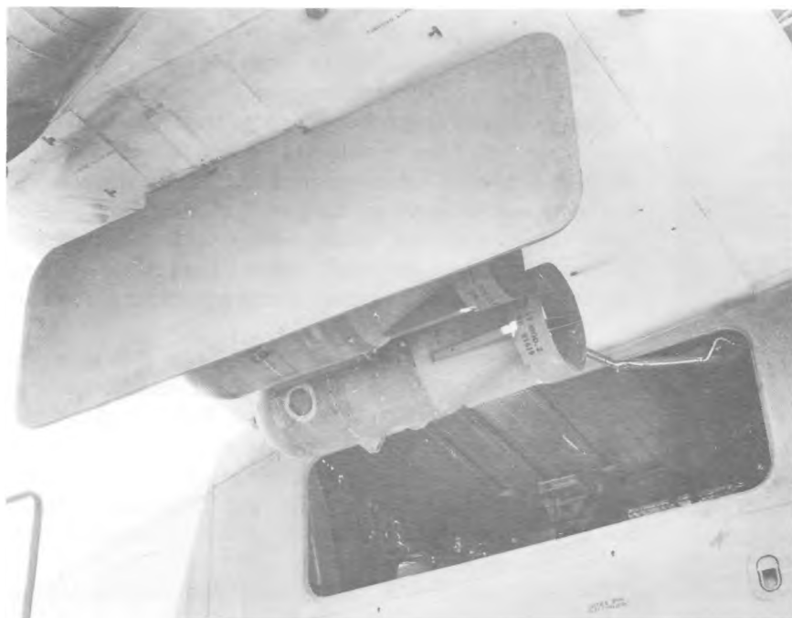
Port side bomb cart in ready position under left wing. The bomb door was an integral part of the cart. One torpedo (Mk. 13 Mod 1 or 2) could be carried below each wing, between the bomb cart tracks and the respective engine nacelle. The outline of the flight deck escape hatch is visible forward of the bomb door. (National Archives 72-AC-66B-34/Consolidated C31-309)
