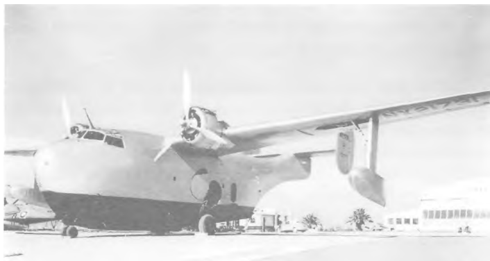
The Model 31 in early April 1941. The straight spine has been replaced by an upward-swept afterbody, and a new mooring hatch has been added to the nose below the flight deck.
