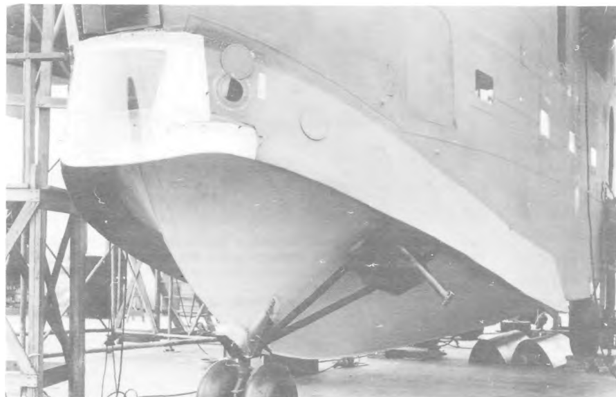
Detail view of lower nose and left forebody of the hull, showing nose gunner's aiming window; flared skirt on hull; open bomb door, main entrance door, and flight deck escape hatch. The forward (nose) beaching gear is installed.
