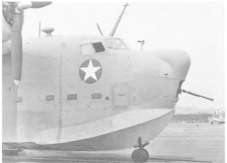
Exterior right nose view, showing radome, cannon, radio antennae masts, and flared forebody skirt. (National Archives 72-AC-66B-24/Consolidated C31 -300)
