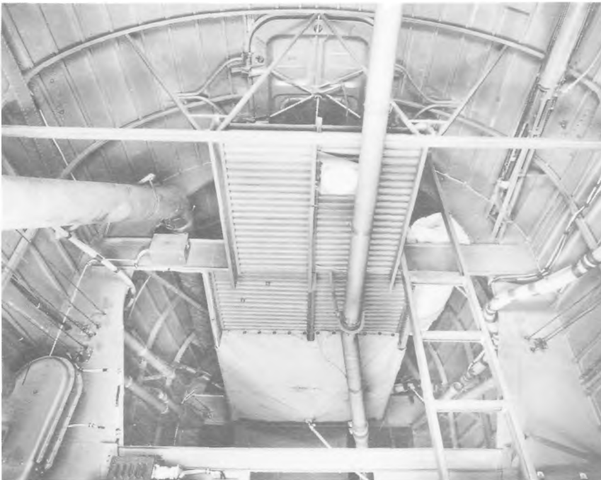
In the waist turret section, amidships, looking aft and up to the main work platform and mid-upper turret. The main entrance door was on the port side of the hull at this point, with an auxiliary power unit to starboard. A large escape hatch is visible above the work platform at the top of the hull.
