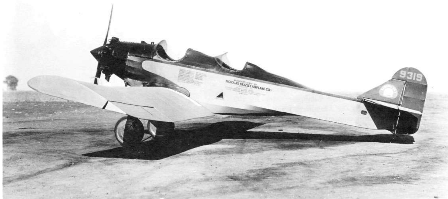
NB-3 C-9319 (No. 21) with a modified and more streamlined nose configuration. The louvered nose cowl and the location of the oil and fuel tanks further aft is significant. It helped some on the instability problems associated with the NB-3, but did not completely solve them. It is not clear if this design change was completed by Barling, Gazley and LaSha or Tom Kirkup. Barling took all (his) records on the NB-3 when he left and it was a while before Kirkup was able to reconstruct some of the basic information files on the NB-3. Gazley and LaSha probably were instrumental in providing N-B with the engineering support required in some of these changes. (R.B. Nicholas)
