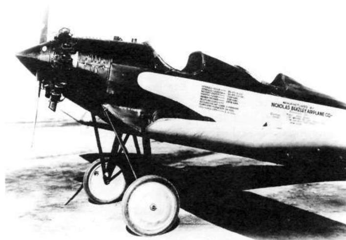
NB-3 C-9319 (No. 21) with a modified and more streamlined nose configuration. The louvered nose cowl and the location of the oil and fuel tanks further aft is significant. It helped some on the instability problems associated with the NB-3, but did not completely solve them. It is not clear if this design change was completed by Barling, Gazley and LaSha or Tom Kirkup. Barling took all (his) records on the NB-3 when he left and it was a while before Kirkup was able to reconstruct some of the basic information files on the NB-3. Gazley and LaSha probably were instrumental in providing N-B with the engineering support required in some of these changes. (R.B. Nicholas)
