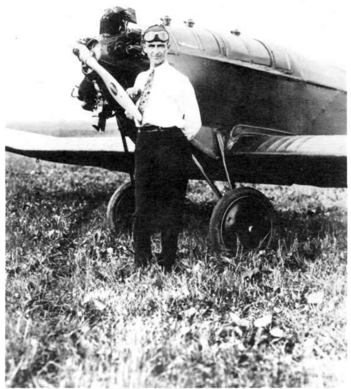
"Barney" Zimmerley with the modified NB-3 used in his 1,600-mile, nonstop flight from Brownsville, Texas, to Winnipeg, Canada. The front cockpit was replaced by an additional fuel tank. The front filler is for an enlarged oil tank. The middle and aft caps are for fuel tanks. The LeBlond engine was later replaced with a Warner Scarab by U.F. Diteman when he purchased this airplane for his ill-fated attempt to fly across the North Atlantic. (R.B. Nicholas)
