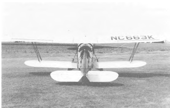
Rear view of the Stearman 4E clearly shows the unequal wingspans that were a characteristic of the early civilian Stearman airplanes. (Kenneth D. Wilson)
