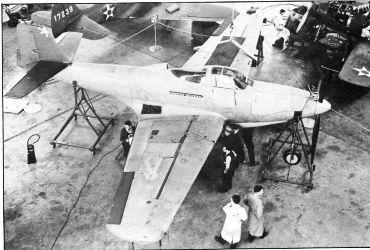
Final assembly photo of what appears to be the first XP-39E (AF41-19501). The singular difference from the wind tunnel model is the use/retention of P-39 wing tips while the squared-off empennage is consistent with the wind tunnel model. (Bell Aerospace via Jay Miller)
