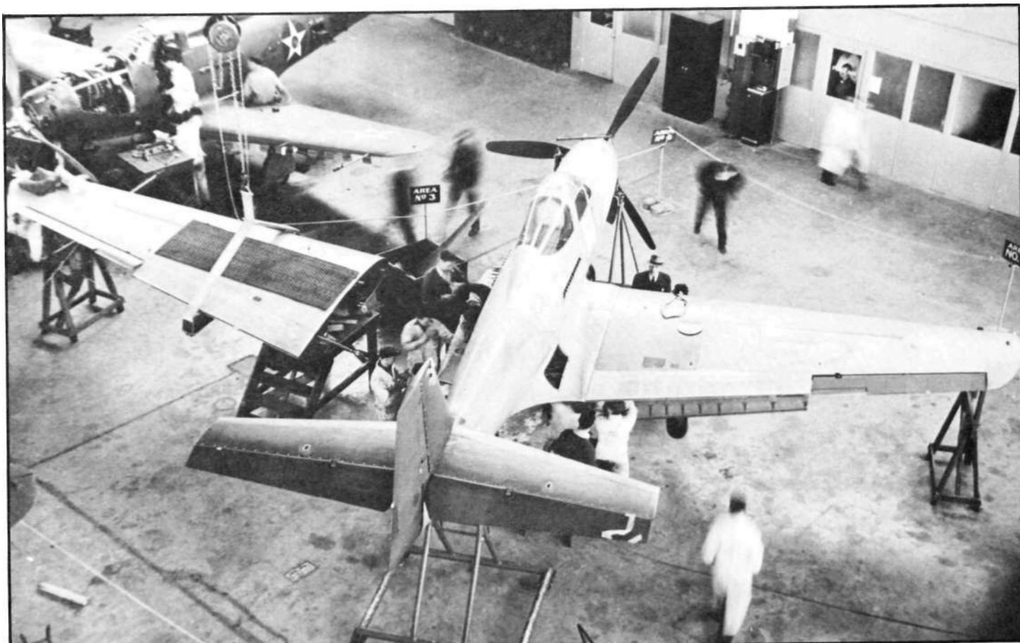
Final assembly photo of what appears to be the first XP-39E (AF41-19501). The singular difference from the wind tunnel model is the use/retention of P-39 wing tips while the squared-off empennage is consistent with the wind tunnel model. (Bell Aerospace via Jay Miller)
