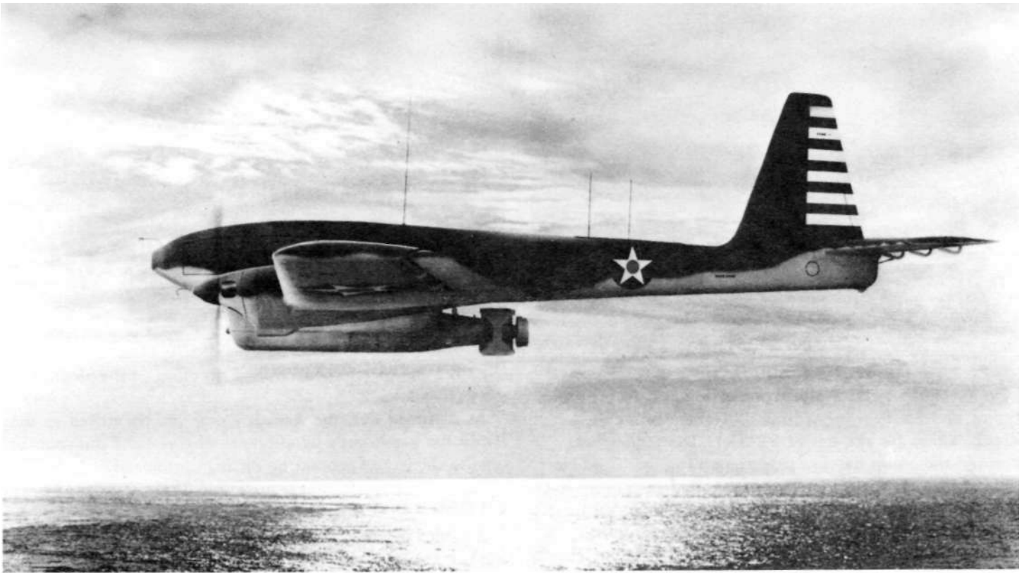
Interstate TDR-1 Assault Drone with torpedo.
