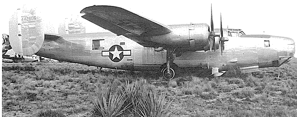
At first glance, this turretless B-24M could be mistaken for a C-109. Note the airfoil-shaped member which is mounted under the belly, just ahead of the bomb bays. This is the long-span antenna of an Eagle bombing radar system. (William T. Larkins photo)
