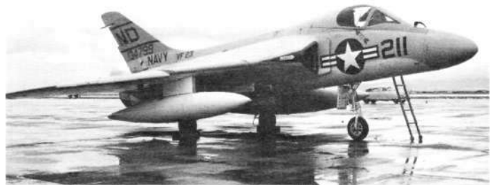
VF-23 Skyrays carried ATG-4's "ND" tail code and the airplane's serial number within the yellow tail band. Note that the national Insignia overlaps onto the intake baffle plate. (William T. Larkins)
