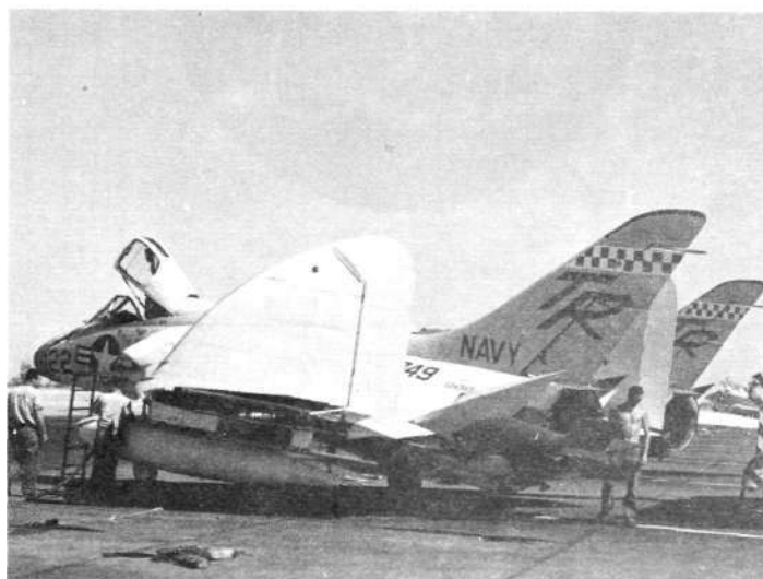
The red and white checkerboard pattern on FAGUPAC Skyrays was eventually reduced to a narrow band on their tails. F4D-1 134749 has the Del Mar high-speed target mounted on left wing. (Navy)
