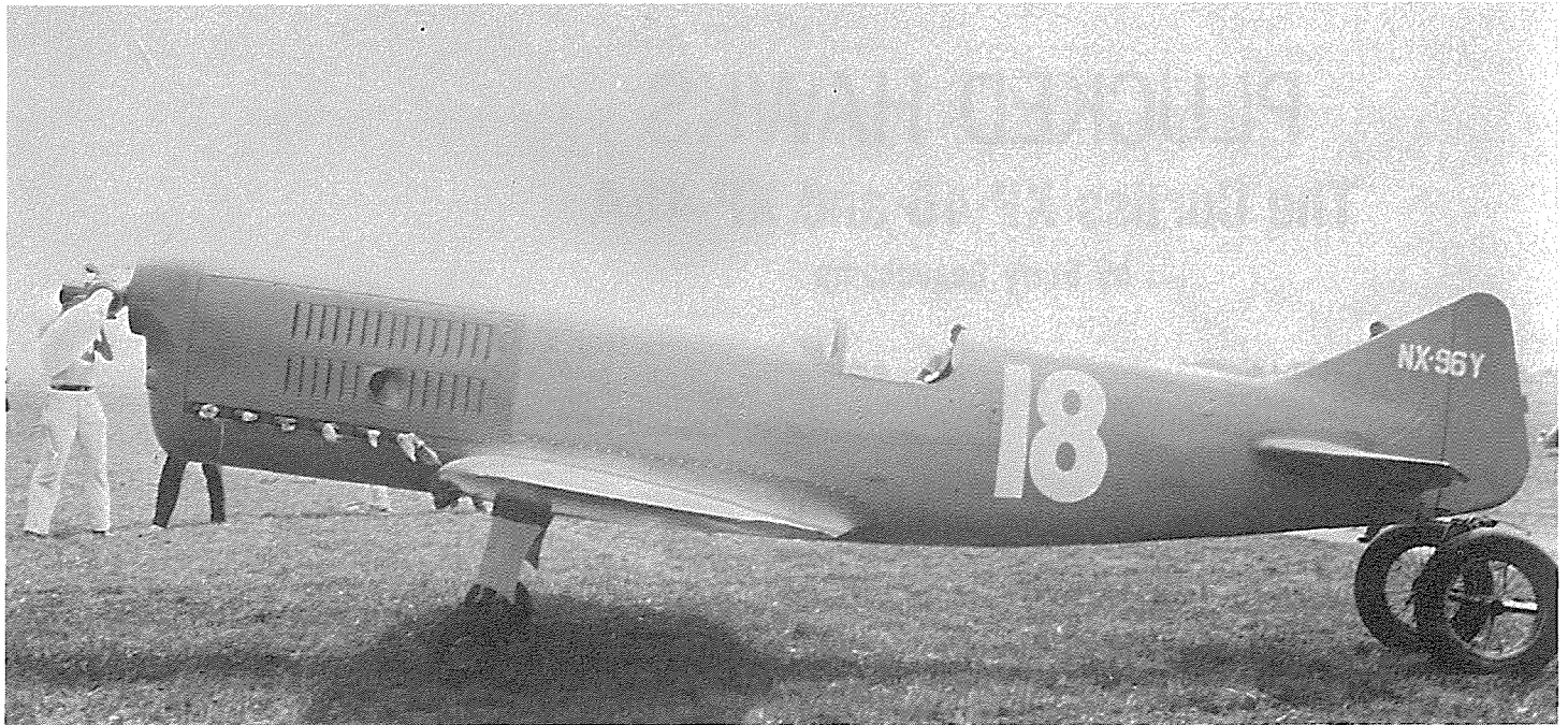
Apparently cooling was still a problem at the races. Note the large opening added to the lower row of louvers.
