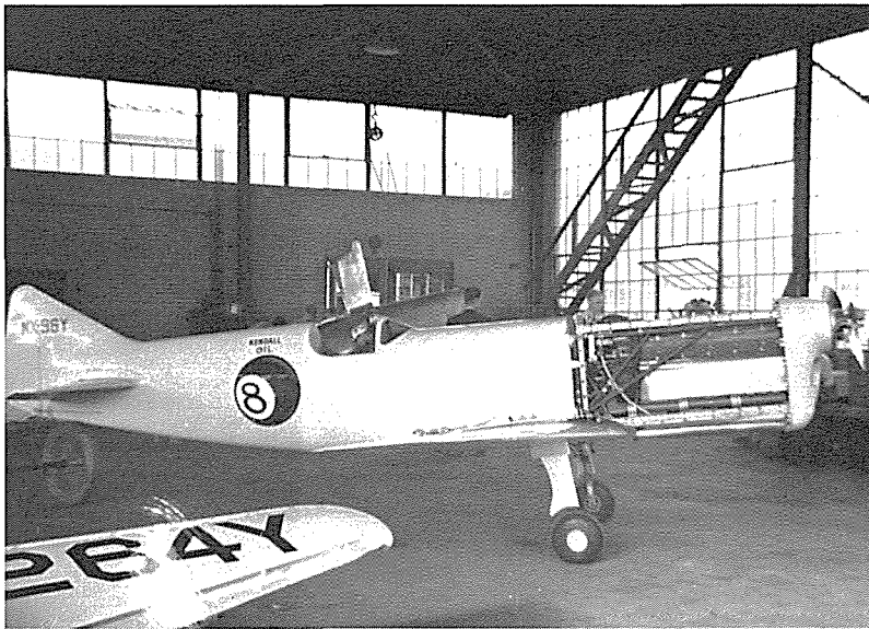
This hangar shot shows the engine installation. The engine bearer can be seen above the engine mounting pads.
