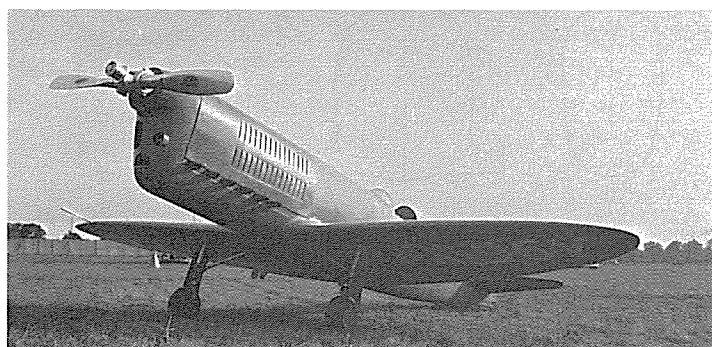
Story-Gawley. Note the louvers on the engine cowl have been nearly removed on the right side of the cowl to improve air cooling of the engine.
