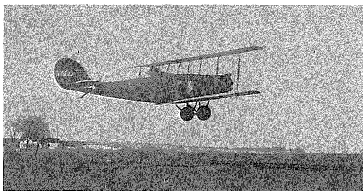
1924—Waco “8”. Color: All silver. Number sold: 1. Liberty “6” 250-hp. Advance Aircraft Co., Troy, Ohio. Cabin held six with two in cockpit. Top speed: 95 mph. Ldg. speed: 37 mph. Brukner flew this plane with six passengers to 1924 Dayton Air Races. Young Paul Westfahl is on the wing walk. (Ray Brantly)
