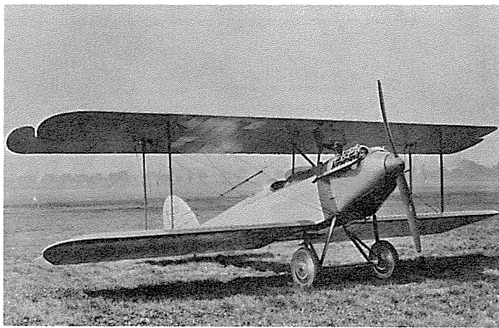
1926—Waco "9" at McCook AFB, Dayton. C/n 30. Color: All silver with maroon cowling. XP 447, Advance Aircraft Co., Troy, Ohio. One of two models purchased from Embry-Riddle by Army Air Corps (A.C. 26-206) for first stress tests to qualify for ATC#11. (Ray Brandy)
