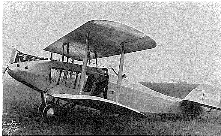
1924—Waco “8”. Color: All silver. Number sold: 1. Liberty “6” 250-hp. Advance Aircraft Co., Troy, Ohio. Cabin held six with two in cockpit. Top speed: 95 mph. Ldg. speed: 37 mph. Brukner flew this plane with six passengers to 1924 Dayton Air Races. Young Paul Westfahl is on the wing walk. (Ray Brantly)
