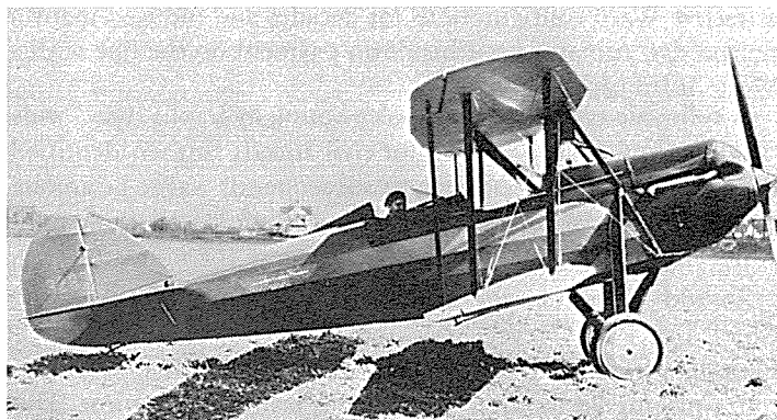
March 30, 1927—Waco "10" No. 3287, Park Board Field, Troy, Ohio (OX-5 90-hp). Shown with the first set of tapered wings installed on a stock Model "10" for test purposes. Outstanding results led to design of aerobatically famous Taperwing. (Ray Brandy)
