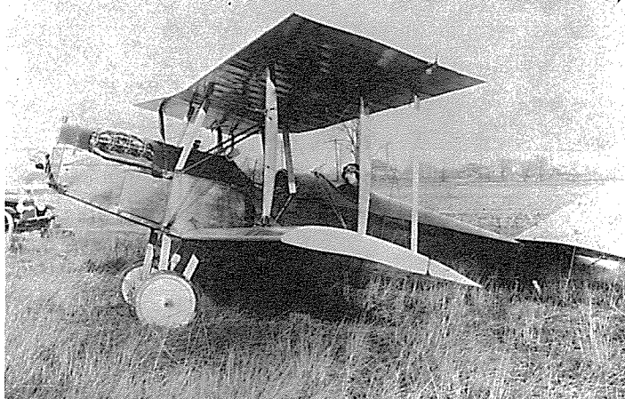
1920—Waco "4". Weaver Aircraft Co., Lorain, Ohio. Color: Fuselage natural finish mahogany plywood. Fabric clear doped. No. sold: 1. OX-5 90-hp, four-place (3 in front cockpit). Utilized modified "Jenny" surplus parts. First passenger-carrying biplane. (James C. Kessler)
