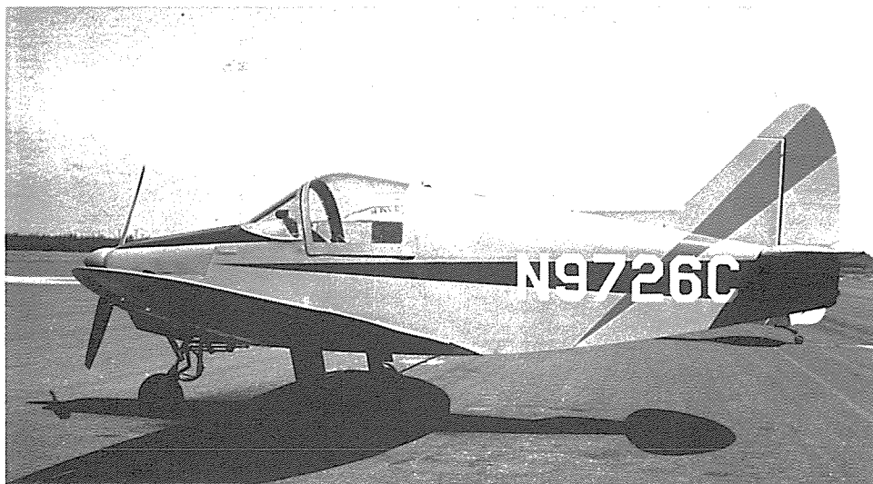
Final configuration of prototype LARK-95 showing plywood and fibreglas-covered wings, fibreglas cowl, revised hatch, and chrome yellow paint with brown and orange stripes.
