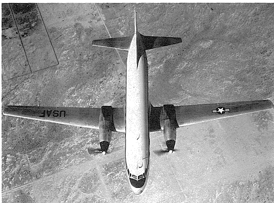
YC-131C 53-7886 showing lengthened horizontal stabilizers and exhaust outlets for YT-56 engines. (Convair N36291 via Charles E. Stewart)
