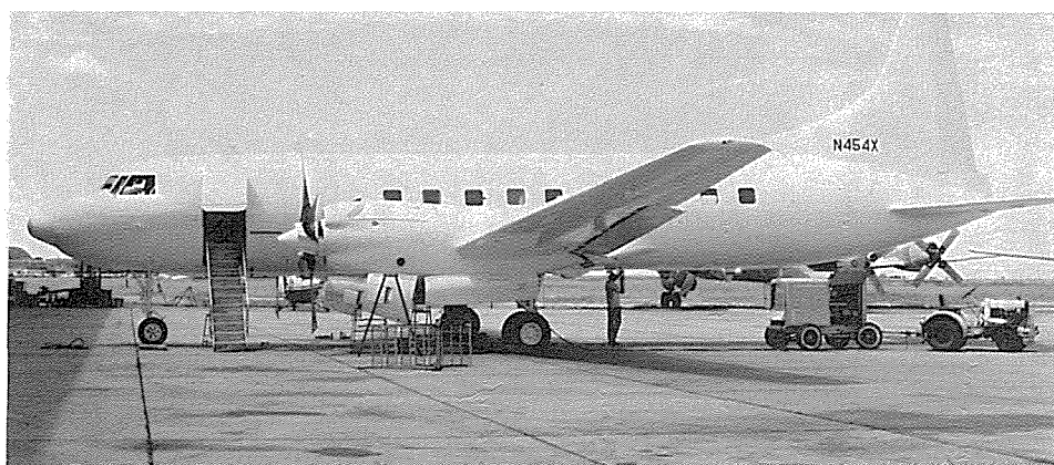
YC-131C 53-7886 was purchased from the FAA by Texas Sun Beechcraft and converted to a Convair 580, although its designation is reportedly "CV-770." Note new nose radar installation in this July 1970 photo, and "experimental" stenciled by doorway of N454X. (Bob Garrard via Ted Gibson)
