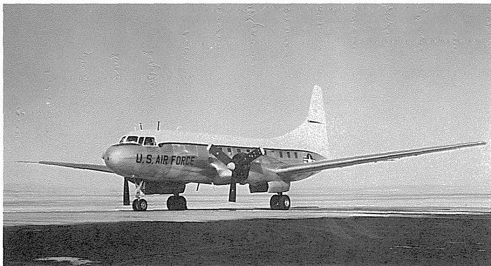
YC-131C 53-7887 at Edwards AFB, California, for safety flight tests. Note wingtip pitot tube. (Air Force K9724)
