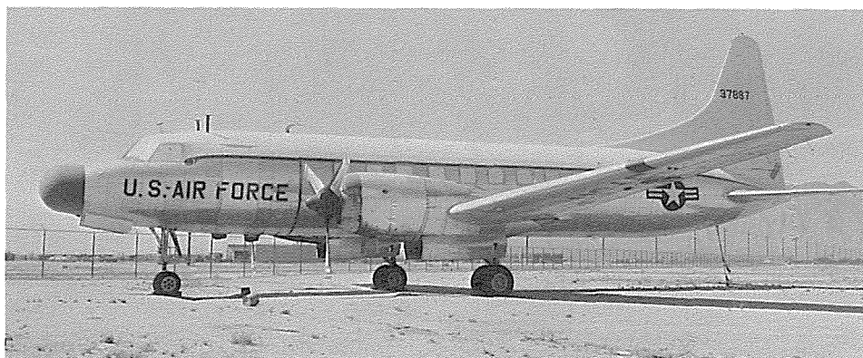
YC-131C 53-7887 at Davis-Monthan AFB in April 1961 shortly before its transfer to the Federal Aviation Agency. This airplane retained its T-56 engines while undergoing extensive nose radar modifications. (Douglas D. Olson)
