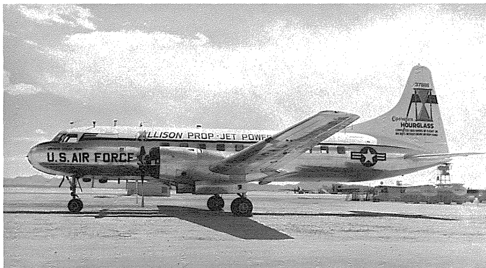
Convair YC-131C 53-7886 at McCarran Field, Las Vegas, Nevada, in April 1958 after completion of "Operation Hourglass" with 3,750 eshp Allison 501-D13 turboprop engines and Aeroproducts propellers. (Paul Stevens)
