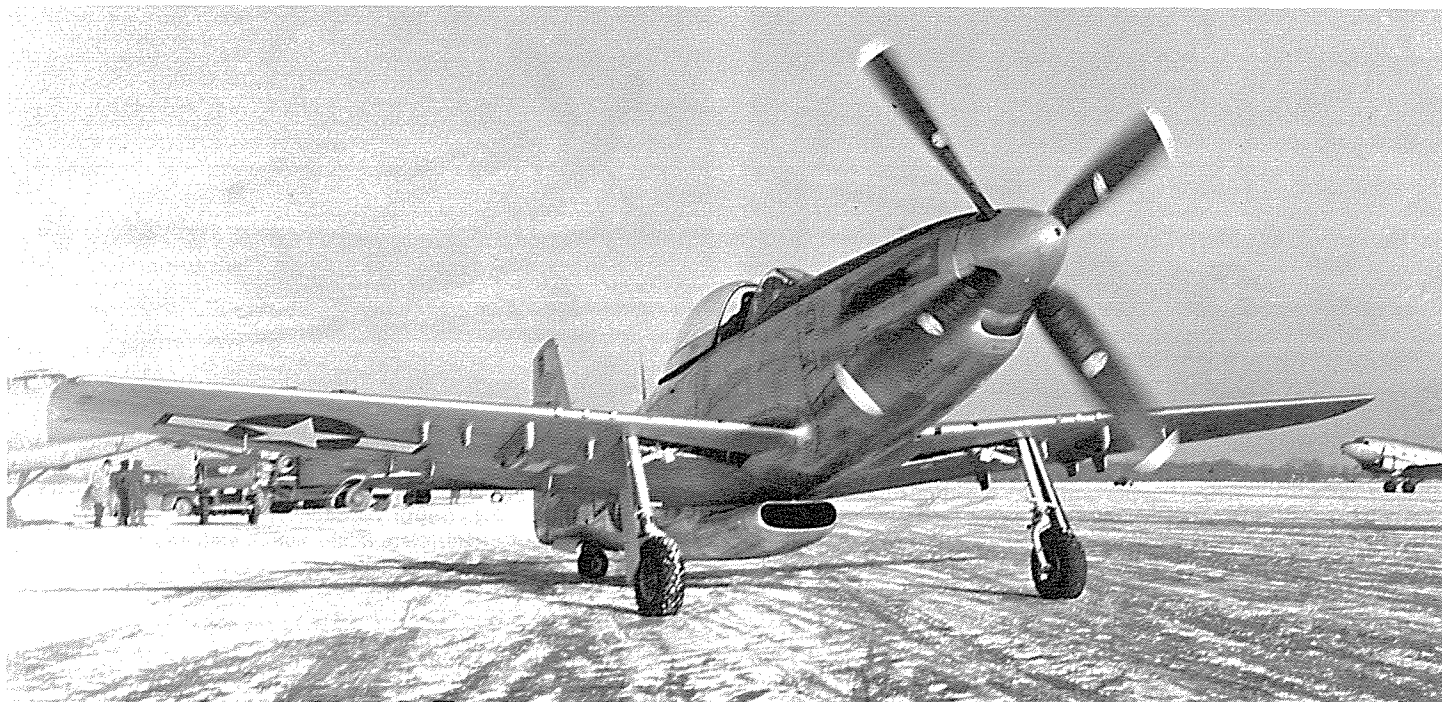
44-64266: Engine run-up at Ft. Dix, NJ. This aircraft has been shown in many publications with a different viewpoint when its cowlings and fuselage were streaked with oil; tracings still being visible in this photograph. Observe that it still is fitted with the interim fin, photographed in Dec. 1945. (AAHS Photo)
