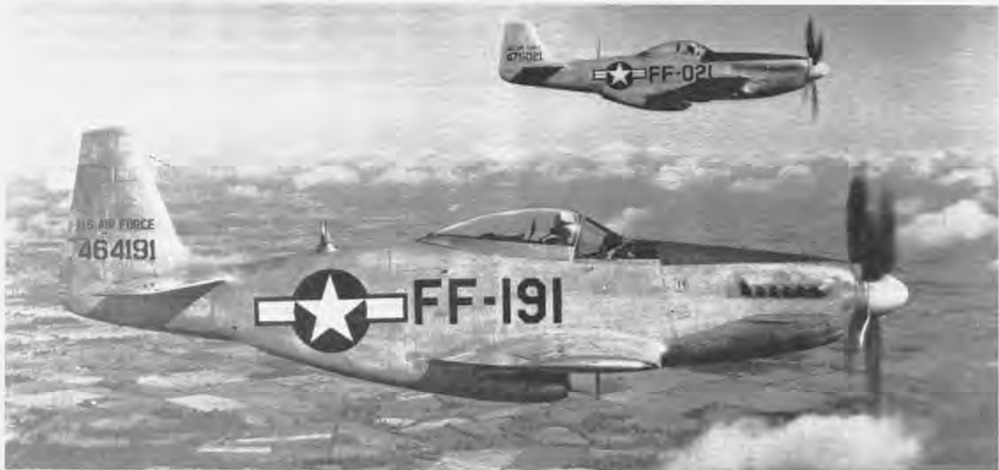
P-51H, 44-64191, and P-51D, 44-75021, demonstrate the design differences between the two models. 191 was wrecked in a takeoff accident in 1954 after accumulating 2,081 hours. (AAHS lending library 7403 via E.C. Carey)
