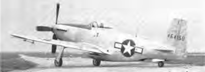
P-51H, 44-64160, with test pitot installation under left wing. This airplane was delivered to the joint Army Air Force/North American Flight Test Division on Jan. 1, 1945. It never became a squadron assigned aircraft. (NAA 126-0-2C courtesy of Dustin Carter) The most photographed P-51H, 44-64164, was delivered to Moffett
