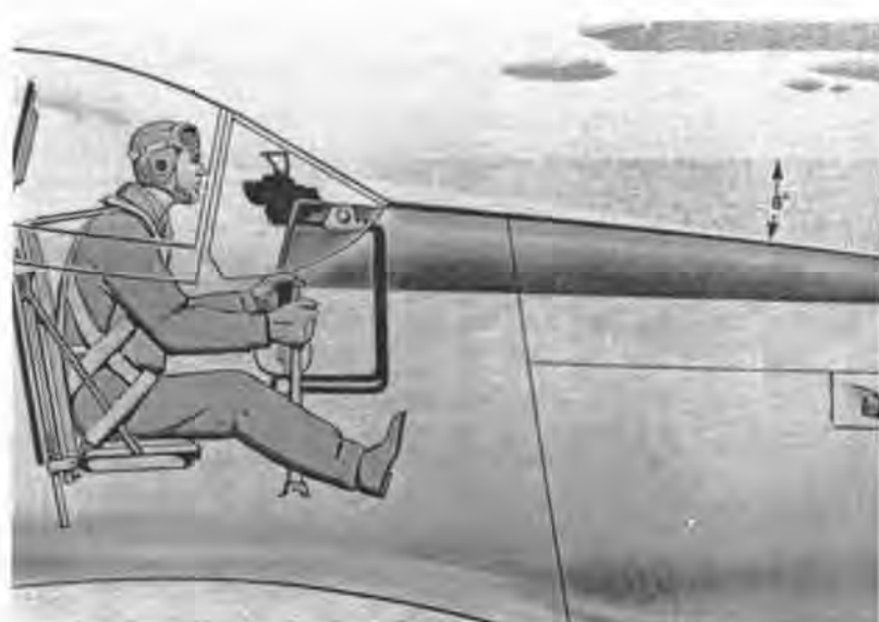
The P-51H's revised engine cowling enhanced target acquisition and deflection sighting over the nose. The gunsight's range compensating unit was built into the throttle. (Author's collection)
