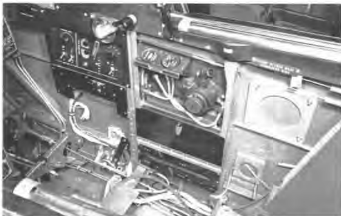
Right side of cockpit of P-51H showing IFF panel and oxygen system indicators. (NAA 126-30-2B courtesy of G.H. Balzer)
