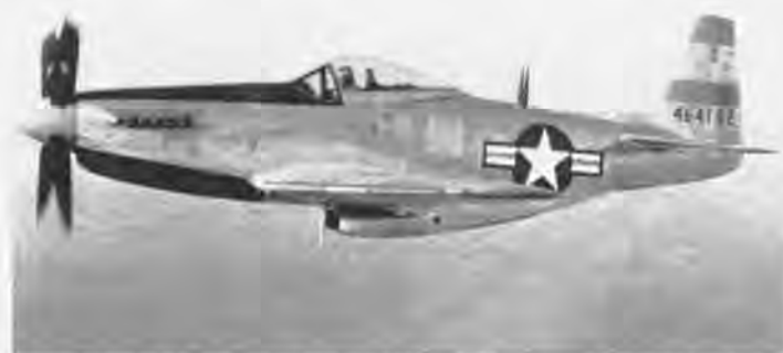
P-51H, Navy BuAer 09064, being flown by Lt. K. Kulig near Grumman Field, Long Island, New York. Note additional pitot tube under left wing and modification made to leading edge of wing. The 82nd Fighter Group field number "60" has been removed from the fin cap, as well as the airplane's data block. (Roger Besecker collection)
