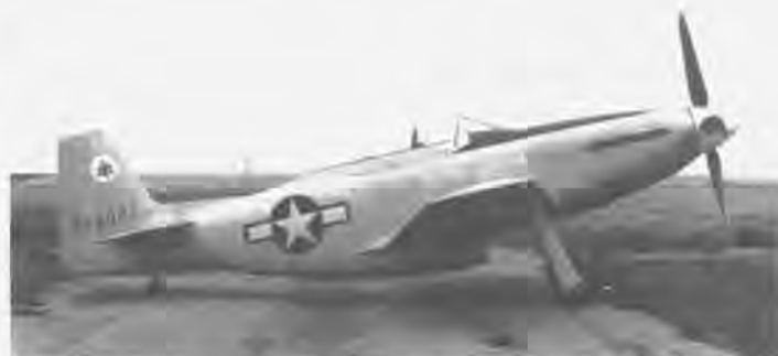
The XP-51J, 44-76027, probably the cleanest looking Mustang with its tightly cowled Allison engine. (NAA 105B-0-33)
