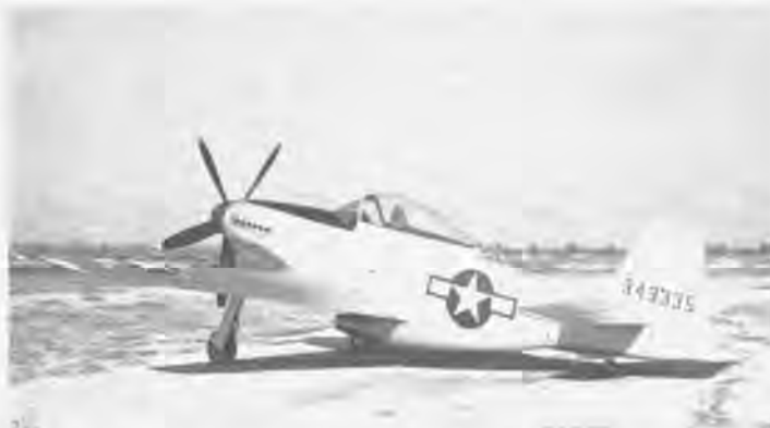
The XP-51G, 43-43335, with a five-bladed prop, was pretty, but the propeller created unworkable difficulties for the plane. (NAA 105A-0-24)
