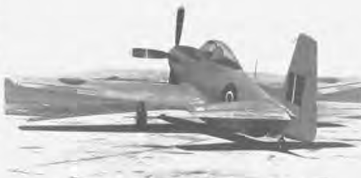
The second XP-51G, 43-43336, in RAF markings. From this angle the rudder appears taller, but was still the P-51D type. (NAA 105A-0-31)
