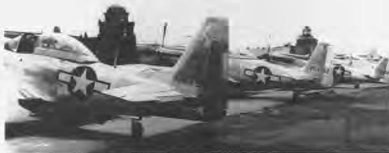
square feet more area than that of production P-51Ds, but it is not the revised P-51H rudder either. The trim tab's top edge is parallel with the balance arm whereas the P-51H's tab was lowered almost a foot. (NAA 122-23-1A)
