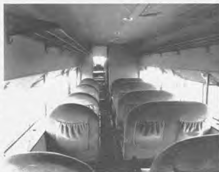
Cabin interior of the prototype Patrician. Snap-shut panels in overhead upholstery conceal emergency exits. Large instruments at upper right of the bulkhead inform passengers of airspeed, altitude and time. (Smithsonian A-2046)
