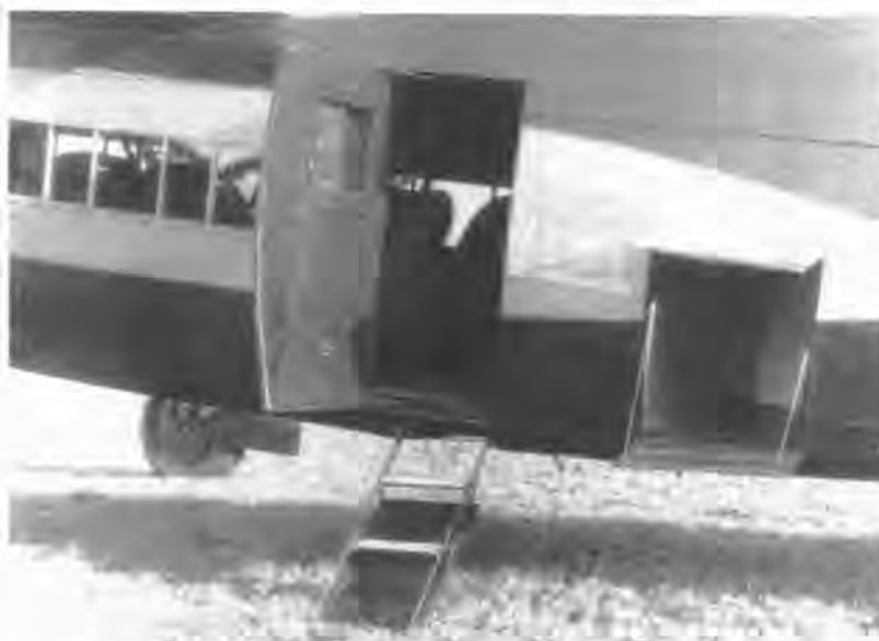
Left side view of the prototype Patrician showing integral boarding steps which could be stowed beneath the cabin floor when not in use. (Smithsonian 76-16775)
