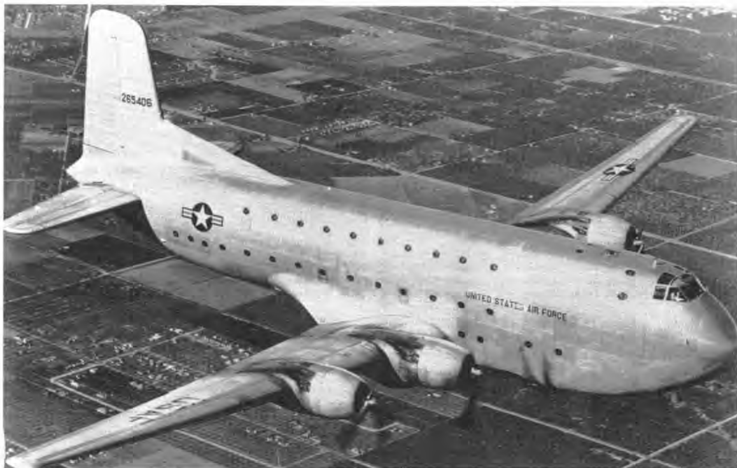
YC-124A, 42-65406, after being converted from C-74, was tested for four years, re-engined with R-4360-35As, and redesignated YC-124C. (Air Force 39685 AC courtesy of Air Force Museum)
