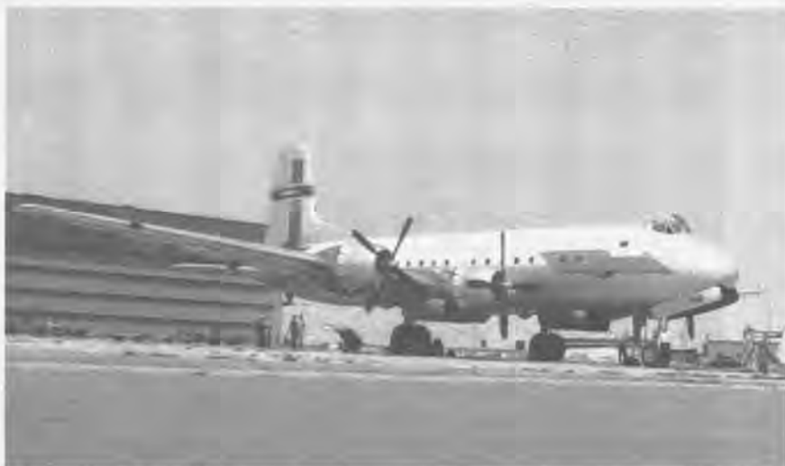
MATS applied a sun-reflective white paint to most C-74s during their later years, as shown by 42-65413 at the Douglas Long Beach plant in May 1955. (Douglas C28707-12)
