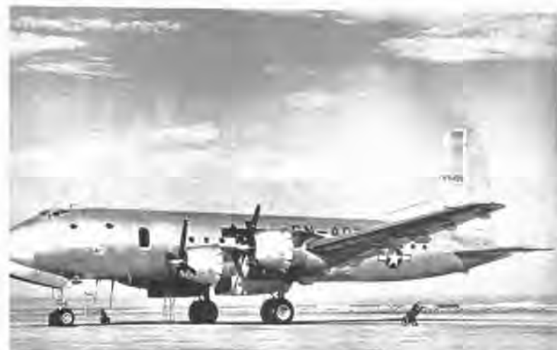
The ill-fated second C-74, 42-65403, at Muroc Army Air Base early in 1946. Note flight test pitot tube on wing and photo reference marks on fuselage. (Douglas via Harry Gann)
