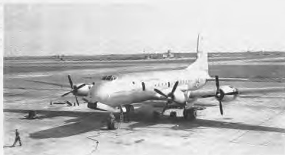
Globemaster to be modified with a new "greenhouse" canopy. Long Beach Airport in the background. (Douglas C 20444-3)
