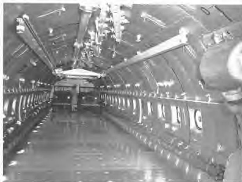
The main cabin of the C-74 was 75 feet long and had a 6,800-cubic-foot capacity. Twin electric cranes rode on overhead rails. The cargo elevator is in front of Jeeps. (Douglas by Lawrence Kronquist)
