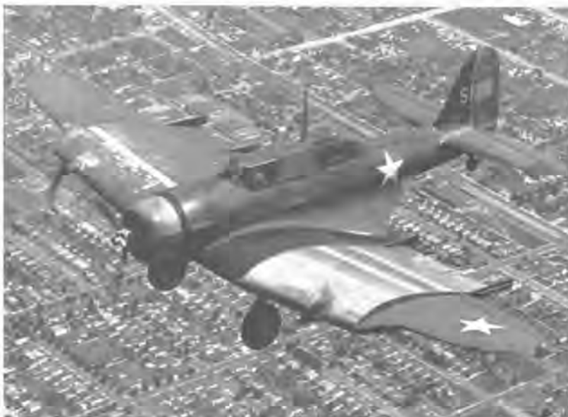
Northrop A-17, 35-122, fitted with wing gloves which simulated the C-74 wing section. Leading edge propellers were free turning. (Douglas via Harry Gann)
