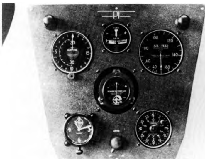
Pilot's instruments. Instrumentation for earth inductor compass consists of dial to be set for proper course at lower right and "On Course" indicator at center.
