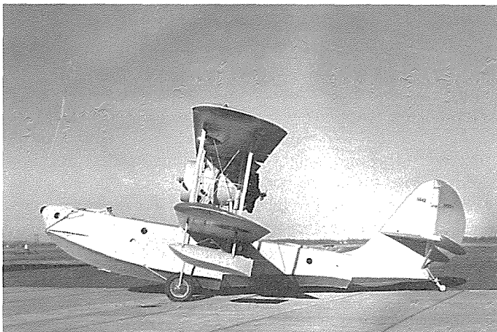
Sikorsky XP2S-1. A U.S. Navy design, engineered and built by Sikorsky, underwent considerable development between 1930 when it appeared powered by two 300 hp P&WA Wasp, Jr. engines and 1932 when the airplane was rebuilt with two 420 hp P&WA Wasp C engines as shown. Only one was built and did not go into production. (United Technologies Archives)
