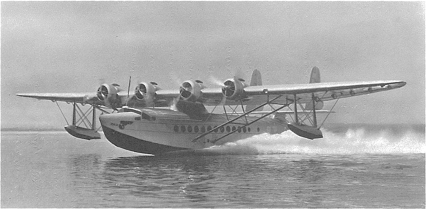
Sikorsky S-42's superior hull design enabled a 35-second takeoff with full load in a dead calm. (United Technologies Archives)
