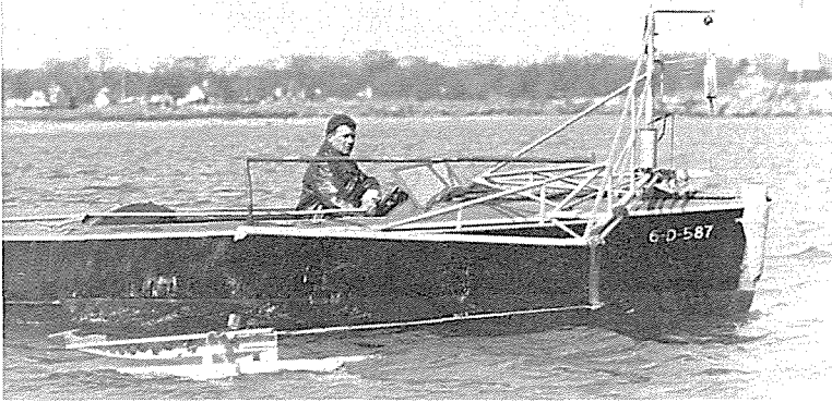
Sikorsky hull model tow test apparatus. A special planning motor boat equipped with a steel tube model supporting boom, instrumen-
