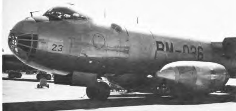
Special engine-carrying "pods" installed on test plane 44-92026. These were the type of pods used on Lt. Col. John D. Bartlett's B-36 to carry spare engines on the June 19, 1950, long-distance flight. (General Dynamics, Fort Worth)
