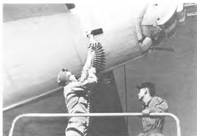
Munitions personnel load the tail stinger of a B-36. Each gun carried 600 rounds of ammo with the exception of the nose turret guns which had only 400 rounds each. (USAF via David A. Anderton)
