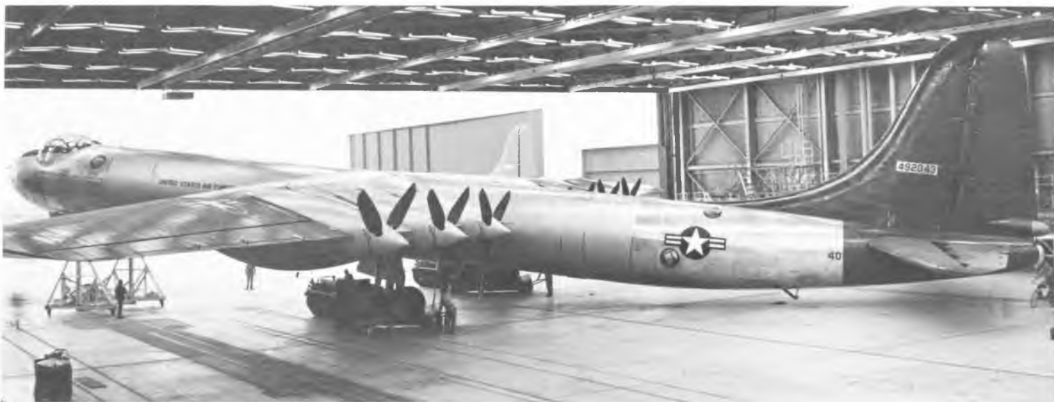
Red-tailed B-36B, 44-92043, being rolled out of the factory. Notice dull magnesium center fuselage compared to nose and rear fuselage sections. (General Dynamics, Fort Worth)
