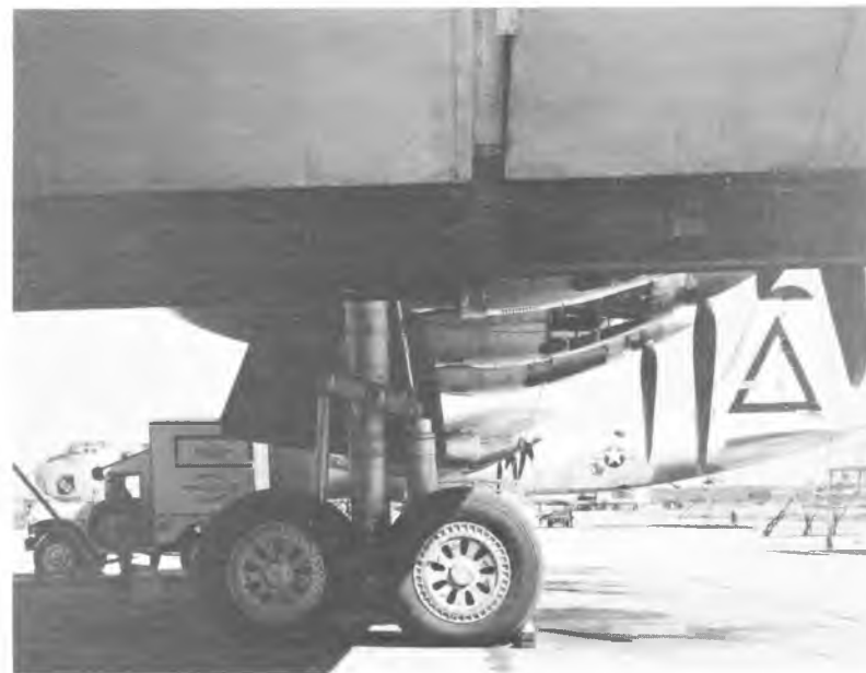
B-36B, 44-92077, framed by another 7th Bomb Wing B-36. Notice sliding panel roll-type bomb bay doors, later to be modified to quicker snap-action hydraulic doors. (RKO Radio Pictures via Walter Jefferies)
