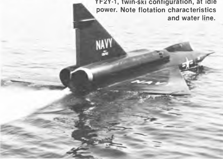
The XF2Y-1 was refitted with the more powerful J-46 Westinghouse engines and continued to be used as the primary testbed for twin-ski changes until mid-1954 when it was converted to the single-ski configuration.
