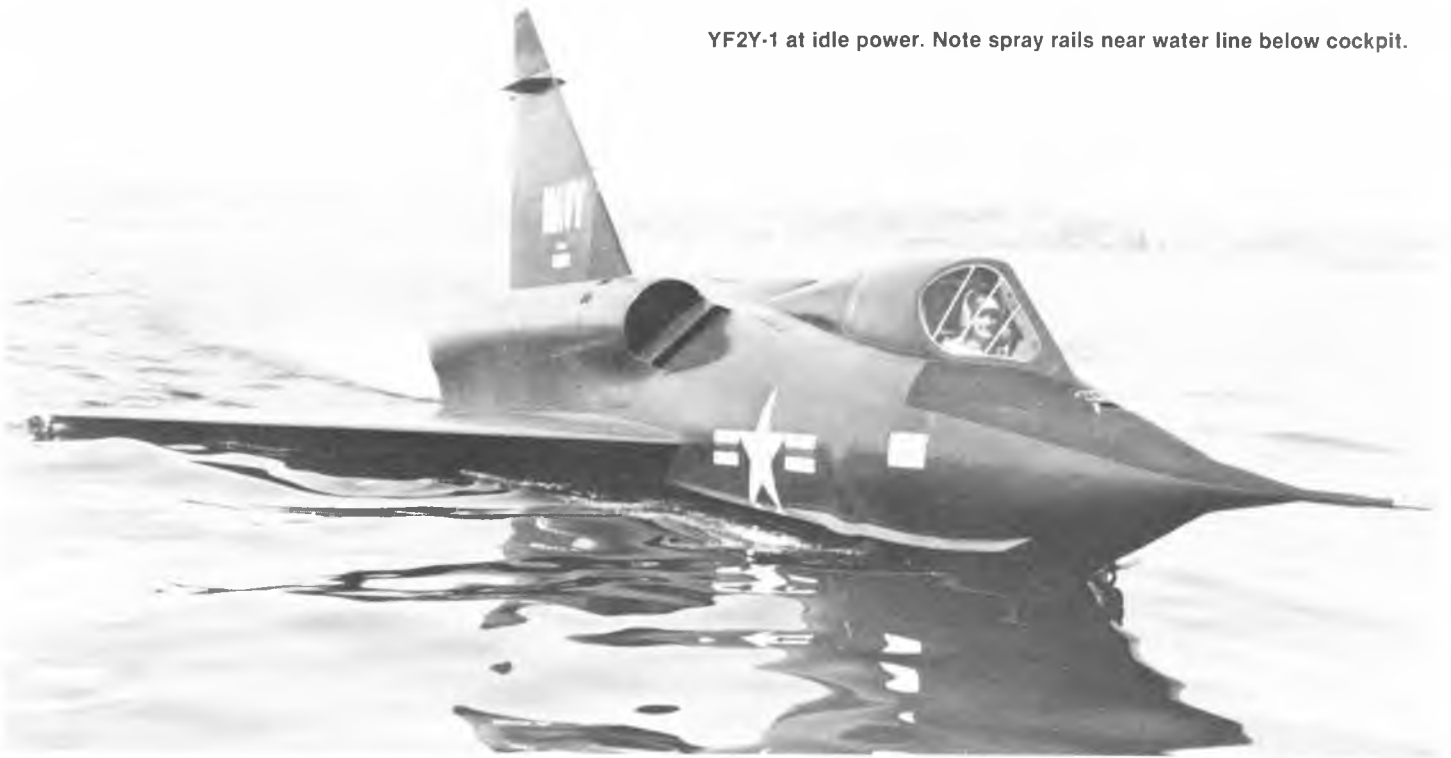
YF2Y-1, twin-ski configuration, at idle power. Note flotation characteristics and water line.
