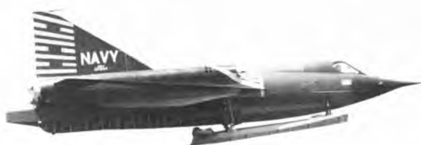
XF2Y-1 with single ski in "stowed" position during slow cruise to open sea test site. This hydrodynamic test configuration was not made fully retractable. Note beaching wheels in retracted position.
