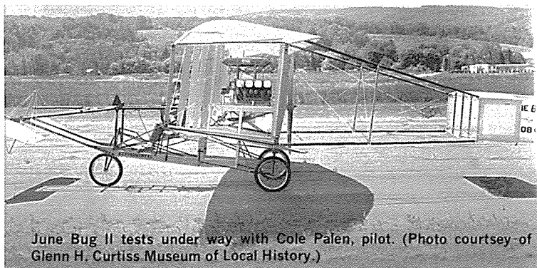
Hammondsport, NY, June 23, 1976—June Bug II with end cells of horiz. stabilizer removed for more effective rudder control. Note vertical trim tab on L.H. end of horiz. stabilizer. (Courtesy Steven Havill)
