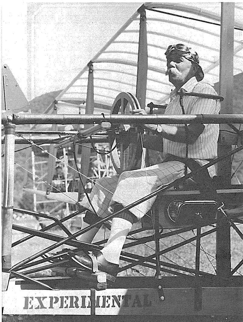
David Fox in the "cockpit." Vane airspeed indicator located on left forward tubular support. Control wheel has rear rudder control wires, engine controls — connected to "push pull" fwd elevator (foot stirrups nonfunctional). Tachometer and oil pressure instruments on left side of seat are read from mirror image. Shoulder yoke controls tip ailerons. Fox is wearing Early Bird cap loaned by Smithsonian's Louis Casey. Bamboo exterior tubing houses inner steel tubing structure. (Courtesy Mike Mandiak)
