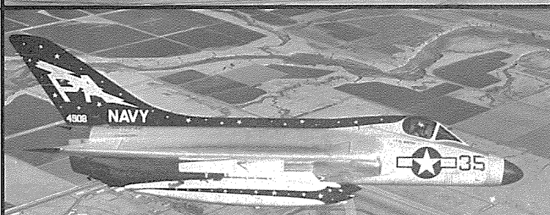
One of two new marking schemes seen on FAWTUPAC Skyrays at the Third Annual Air Weapons Meet at NAAS El Centro in April 1958. Dark insignia blue - spine, tail, and drop tanks; yellow - stars and lightning bolt; white - lettering on tail. (US Navy).
